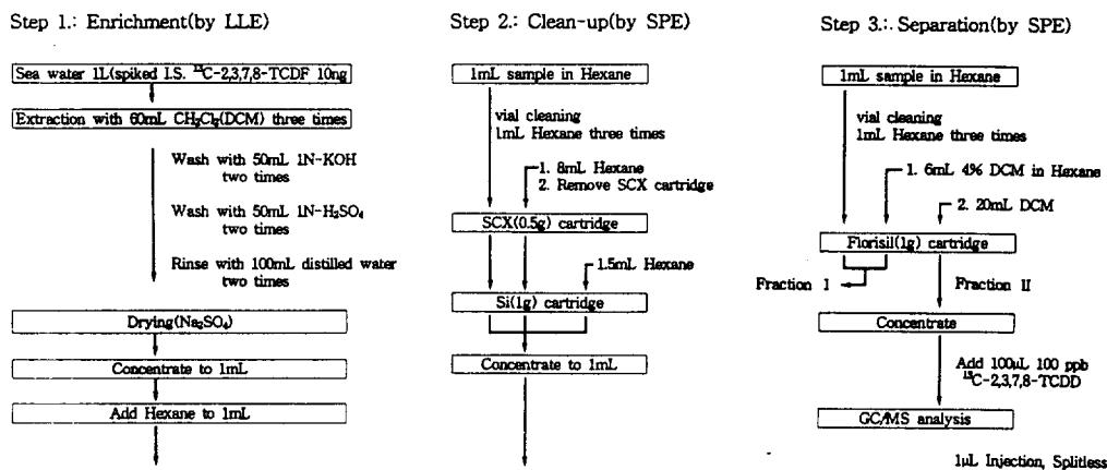
Fig. 2. Experimental procedure of sample pretreatment.
