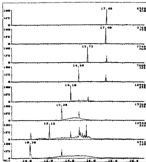
Fig. 4. GC/MS chromatogram of fraction of 6 ml 4% DCM/Hexane in Florisil separation procedure. Peak I.D., 10.30 (retention time) : 2-Monochlorinated biphenyl, 12.12 : 2,3-Dichlorinated biphenyl, 13.28 : 2,4,5-Trichlorinated biphenyl, 14.10 : 2,2',4,4'-Tetrachlorinated biphenyl, 14.88 : 2,2',3',4,6-Pentachlorinated biphenyl, 15.73 : 2,2',4,4',5,6'-Hexachlorinated biphenyl, 17.40 : 2,2',3,3',4,4',6-Heptachlorinated biphenyl, 17.48 : 2,2',3,3',4,5',6,6'-Octachlorinated biphenyl.
