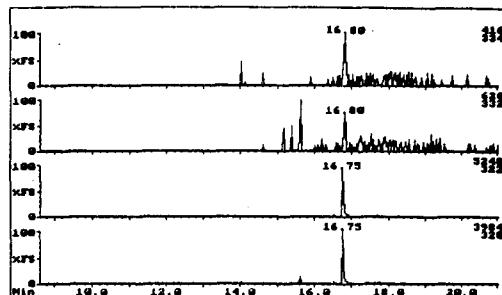
Fig. 5. GC/MS chromatogram of fraction of 20 ml DCM in Florisil separation procedure. Peak I.D., 16.75 : 1,2,3,4-TCDD, 16.80 :  $^{13}\text{C}$ -2,3,7,8-TCDD.
