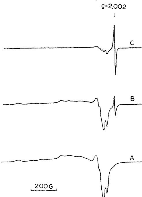
Fig. 2. EPR spectra of Cu(II)Y and effect of furan adsorption. (A) evacuation at 200°C for 4hr. (B) furan on Cu(II)Y. (C) additional furan added to B.
