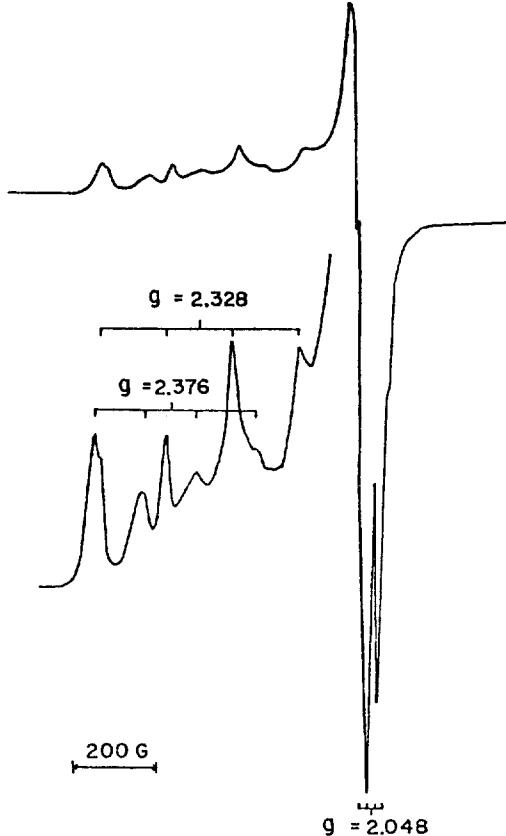
Fig. 1. EPR spectrum of dehydrated  $\text{Cu}(15)\text{Y}$ .
