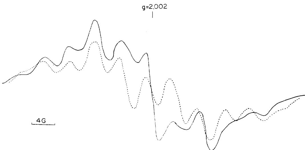
Fig. 4. Expanded (new band portion) EPR spectrum of 2-methylfuran adsorbed on Cu(15)Y.
