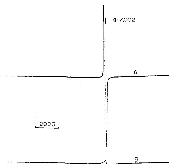
Fig. 3. EPR spectra of Cu(15)Y. (A) after the addition of furan and heating to 300°C. (B) after treating A with oxygen at room temperature.
