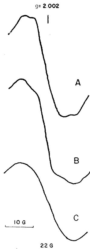
*Fig. 5. Expanded (new band portion) EPR spectra of 2-methylfuran adsorbed on Cu(29)Y-A, Cu(42)Y-B, and Cu(60)Y-C.*
