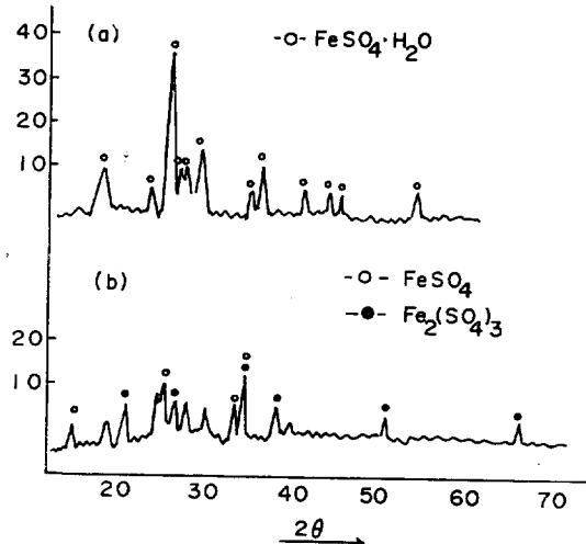
Fig. 2. X-ray diffraction patterns of (a) the sample obtained in DTA at  $300^\circ\text{C}$  and (b) the sample obtained in DTA at  $500^\circ\text{C}$  (CuKa)
