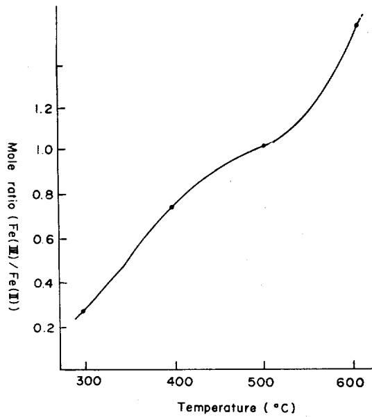
Fig. 4. Plot of mole ratio ( $\text{Fe(III)}/\text{Fe(II)}$ ) vs. treating temperature.
