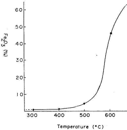
Fig. 3. Plot of  $\text{Fe}_2\text{O}_3$  (%) vs. treating temperature.
