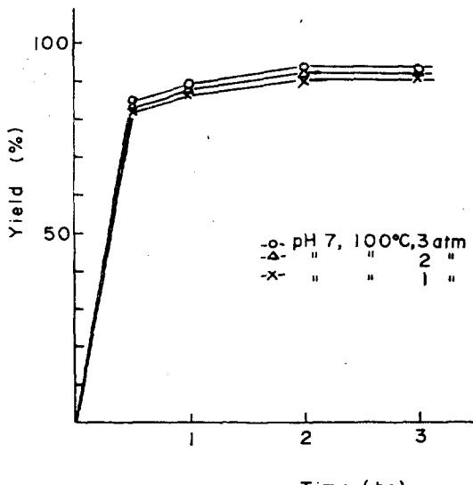
Fig. 5. Yield of  $\alpha\text{-Fe}_3\text{O}_4$  vs. reaction time.
