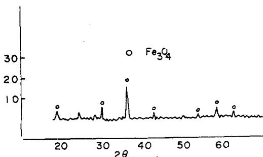
Fig. 6. X-Ray diffraction patterns of  $\alpha\text{-Fe}_3\text{O}_4$  formed ( $\text{CuK}\alpha$ ).
