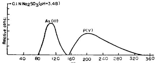
Fig. 2. Elution curves of anion mixture
