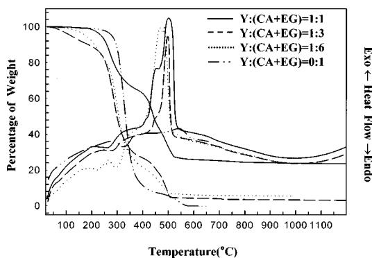
Fig. 2. TG/DTA curve for the preparation of  $\text{Y}_2\text{O}_3$ .
