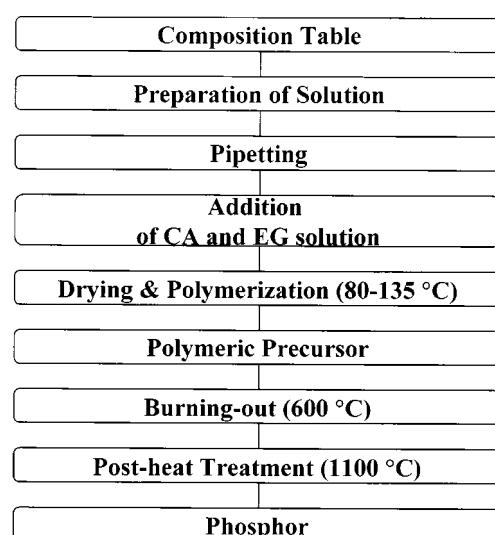
Fig. 1. Flow chart for a polymeric precursor routes.
