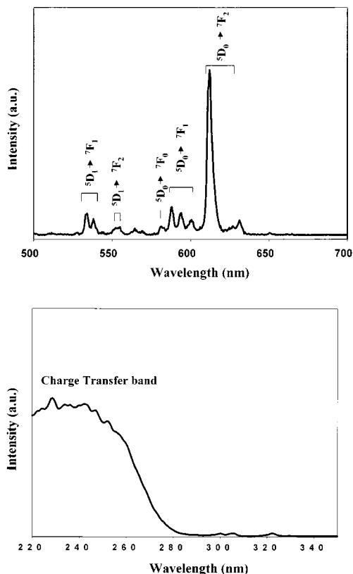
Fig. 3. Excitation and emission spectrum of  $\text{Y}_{(2-x-y)}\text{O}_3$ : Eu<sub>x</sub>, Li<sub>y</sub> (x=0.06 mol, y=0.2 mol).
