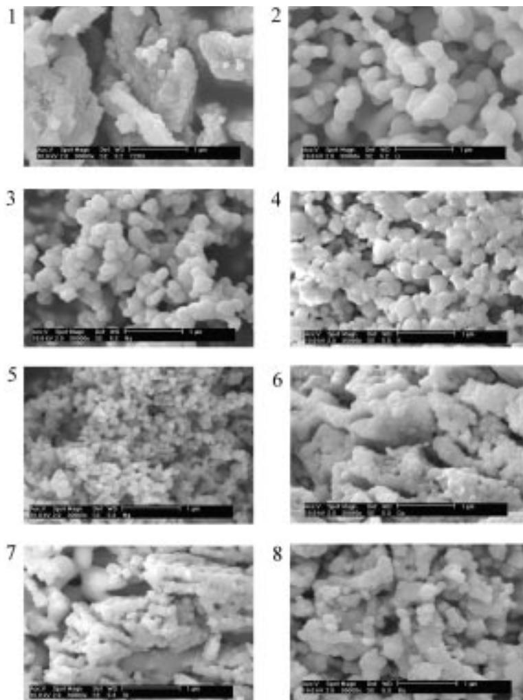
Fig. 5. SEM photographs of  $\text{Y}_{(2-x-y)}\text{O}_3 : \text{Eu}_x, \text{M}_y$  ( $x=0.06 \text{ mol}$ ,  $y=0.2 \text{ mol}$ ) at  $1100^\circ\text{C}$  ① none ② Li ③ Na ④ K ⑤ Mg ⑥ Ca ⑦ Sr ⑧ Ba.
