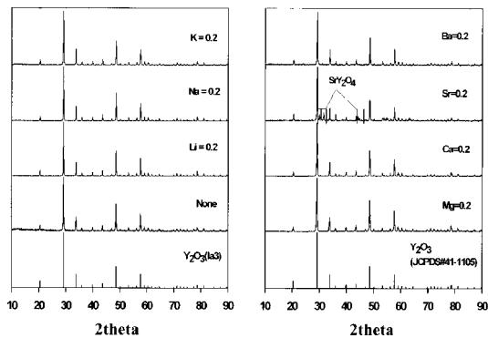
Fig. 4. X-ray diffraction patterns of  $\text{Y}_{(2-x-y)}\text{O}_3$ : Eu<sub>x</sub>, M<sub>y</sub> (x=0.06 mol, y=0.2 mol) at 1100 °C ① none ② Li ③ Na ④ K ⑤ Mg ⑥ Ca ⑦ Sr ⑧ Ba.
