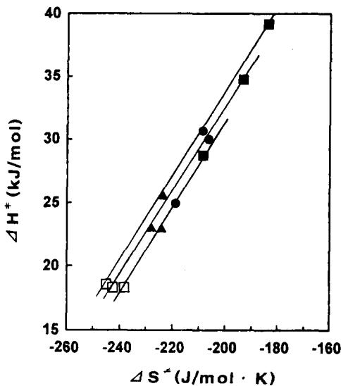
Fig. 3. Isokinetic relations for the reaction of isoquinoline with *para*-substituted benzylbromides in acetonitrile at 25 °C. (■: 1 bar ●: 200 bar ▲: 500 bar ◻: 1000 bar)
