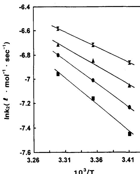
Fig. 2. Arrhenius plots for the reaction of isoquinoline with benzylbromide in the acetonitrile under various pressures. (■: 1 bar ●: 200 bar ▲: 500 bar ✖: 1000 bar)
