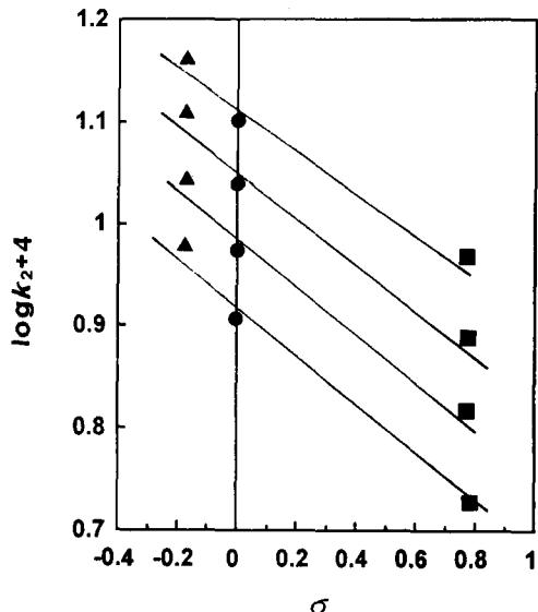
Fig. 4. Hammett plots for the reaction of isoquinoline with *para*-substituted benzylbromide in acetonitrile under various pressures. (■: *p*-NO<sub>2</sub> ●: *p*-H ▲: *p*-CH<sub>3</sub>)
