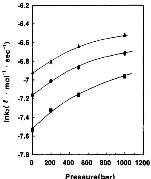
Fig. 1. Pressure dependence of ln k<sub>2</sub> for the reaction of isoquinoline with *para*-substituted benzylbromide in the acetonitrile at 25 °C. (■: *p*-NO<sub>2</sub> ●: *p*-H ▲: *p*-CH<sub>3</sub>)
