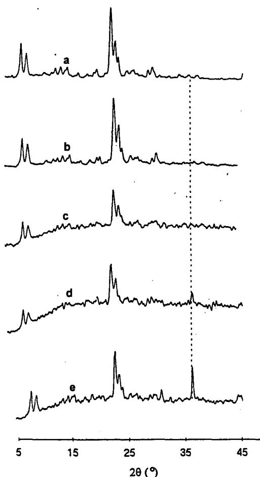
Fig. 4. XRD patterns of (a) HZSM-5, (b) 18 h calcined Co(0.28)/ZSM-5, (c) 1 h calcined Co(3.2)/ZSM-5, (d) 18 h calcined Co(3.2)/ZSM-5 and (e) 19% Co<sub>3</sub>O<sub>4</sub>/ZSM-5.
