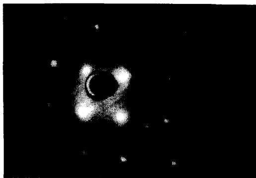
Fig. 5. The LEED pattern obtained from 1 ML Ti/Mo(100) (the electron energy is about 130 eV).
