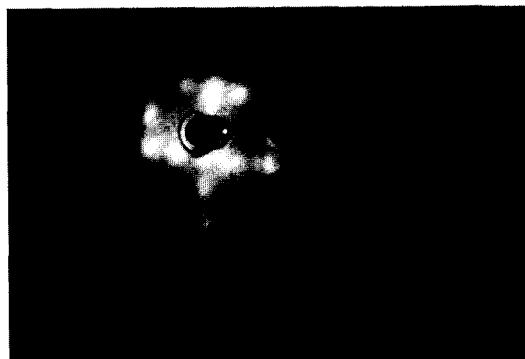
Fig. 8. The LEED pattern for the 30 mL TiO<sub>2</sub>/Mo(100) annealed to 1200K (electron energy is about 95 eV).
