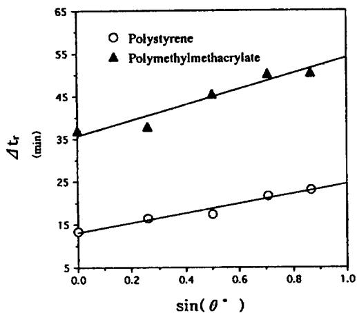
Fig. 13. Retention time difference,  $\Delta t_r$ , vs. thermal FFF system upward angle to horizontal surface for polystyrene and polymethylmethacrylate with different molecular weights in tetrahydrofuran. ps  $\omega = 127 \mu\text{m}$ ;  $\Delta T = 43.5 \text{ K}$ ;  $T_c = 294 \text{ K}$ ; flow = 0.058 mL/min, pmma  $\omega = 127 \mu\text{m}$ ;  $\Delta T = 42 \text{ K}$ ;  $T_c = 296.15 \text{ K}$ ; flow = 0.07 mL/min.
