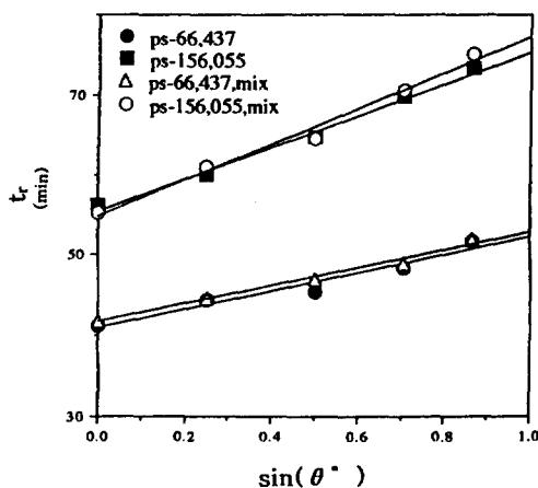
Fig. 10. Retention time,  $t_r$ , vs. thermal FFF system upward angle to horizontal surface for polystyrene with different molecular weights in tetrahydrofuran.  $\omega = 127 \mu\text{m}$ ;  $\Delta T = 43.5 \text{ K}$ ;  $T_c = 294 \text{ K}$ ; flow = 0.058 mL/min.
