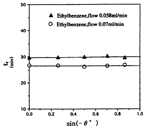
Fig. 5. Retention time,  $t_r$ , vs. thermal FFF system downward angle to horizontal surface for ethylbenzene.  $\omega=127 \mu\text{m}$ ;  $\Delta T=43.5 \text{ K}$ ;  $T_c=294 \text{ K}$ ; flow = 0.058 mL/min,  $\omega=127 \mu\text{m}$ ;  $\Delta T=42 \text{ K}$ ;  $T_c=296.15 \text{ K}$ ; flow = 0.07 mL/min.
