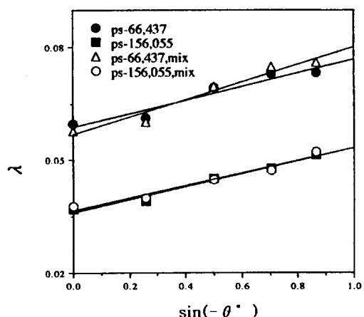
Fig. 7.  $\lambda$  value vs. thermal FFF system downward angle to horizontal surface for polystyrene with different molecular weights in tetrahydrofuran.  $\omega=127 \mu\text{m}$ ;  $\Delta T=43.5 \text{ K}$ ;  $T_c=294 \text{ K}$ ; flow = 0.058 mL/min.
