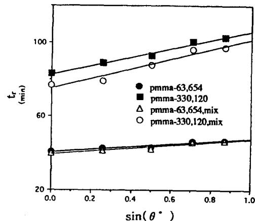
Fig. 11. Retention time,  $t_r$ , vs. thermal FFF system upward angle to horizontal surface for polymethylmethacrylate with different molecular weights in tetrahydrofuran.  $\omega = 127 \mu\text{m}$ ;  $\Delta T = 41 \text{ K}$ ;  $T_c = 297.15 \text{ K}$ ; flow = 0.07 mL/min.
