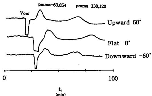
Fig. 15. Retention time difference for downward 60°, 0°, upward 60°, solute = PMMA 63,654 and 330,120 in THF.  $\omega = 127 \mu\text{m}$ ;  $\Delta T = 41.5 \text{ K}$ ;  $T_c = 296.5$ ; flow = 0.07 mL/min.
