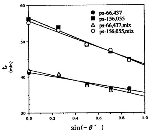
Fig. 6. Retention time,  $t_r$ , vs. thermal FFF system downward angle to horizontal surface for polystyrene with different molecular weights in tetrahydrofuran.  $\omega=127 \mu\text{m}$ ;  $\Delta T=43.5 \text{ K}$ ;  $T_c=294 \text{ K}$ ; flow = 0.058 mL/min.
