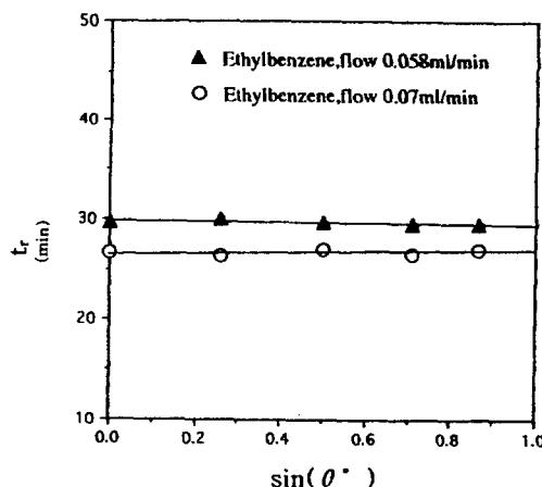
Fig. 9. Retention time,  $t_r$ , vs. thermal FFF system upward angle to horizontal surface for ethylbenzene.  $\omega = 127 \mu\text{m}$ ;  $\Delta T = 43.5 \text{ K}$ ;  $T_c = 294 \text{ K}$ ; flow = 0.058 mL/min,  $\omega = 127 \mu\text{m}$ ;  $\Delta T = 42 \text{ K}$ ;  $T_c = 296.15 \text{ K}$ ; flow = 0.07 mL/min.
