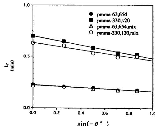
Fig. 8. Retention time,  $t_r$ , vs. thermal FFF system downward angle to horizontal surface for polymethylmethacrylate with different molecular weights in tetrahydrofuran.  $\omega=127 \mu\text{m}$ ;  $\Delta T=42 \text{ K}$ ;  $T_c=296.15 \text{ K}$ ; flow = 0.07 mL/min.
