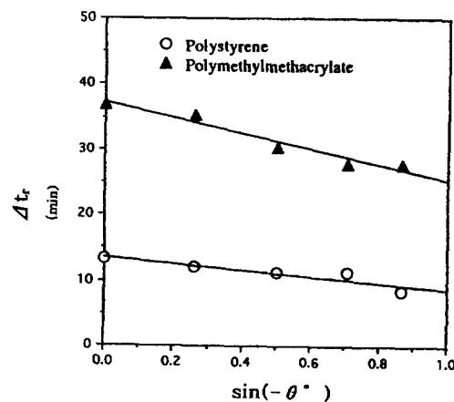
Fig. 12. Retention time difference,  $\Delta t_r$ , vs. thermal FFF system downward angle to horizontal surface for polystyrene and polymethylmethacrylate with different molecular weights in tetrahydrofuran. ps  $\omega = 127 \mu\text{m}$ ;  $\Delta T = 43.5 \text{ K}$ ;  $T_c = 294 \text{ K}$ ; flow = 0.058 mL/min, pmma  $\omega = 127 \mu\text{m}$ ;  $\Delta T = 42 \text{ K}$ ;  $T_c = 296.15 \text{ K}$ ; flow = 0.07 mL/min.
