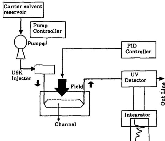
Fig. 2. Schematic diagram of FFF system.
