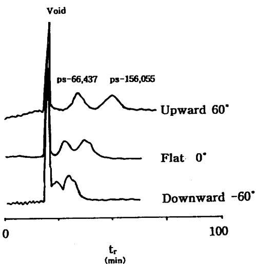
Fig. 14. Retention time difference for downward 60°, 0°, upward 60°, solute = PS 66,437 and 156,055 in THF.  $\omega = 127 \mu\text{m}$ ;  $\Delta T = 43.5 \text{ K}$ ;  $T_c = 294 \text{ K}$ ; flow = 0.058 mL/min.
