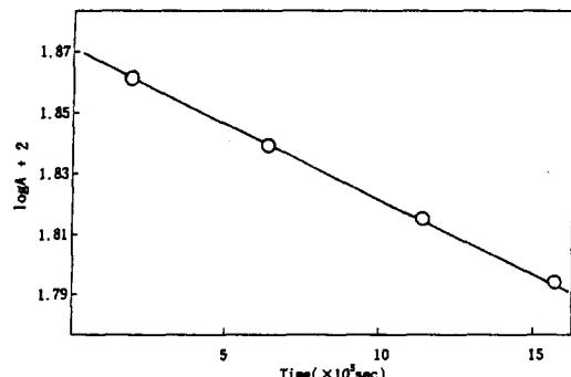
Fig. 1. The plot of log absorbance vs. time for the hydrolysis of 4-acetyl-5,6-dihydro-3-methyl-N-(*p*-chlorophenyl)-1,4-thiazine-2-carboxamide at pH 11.5 and 25°C.
