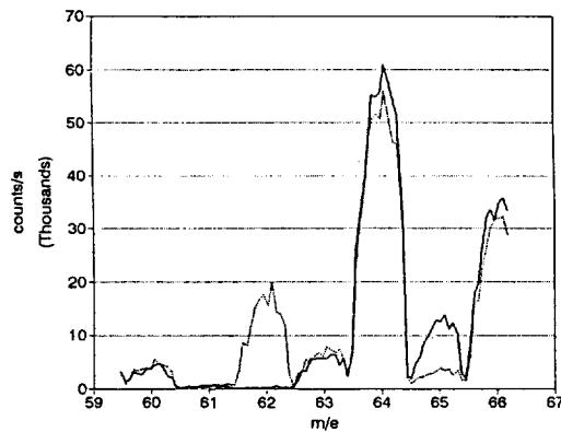
Fig. 4. Ni and Cu isotope peaks illustrating isotope dilution method (dotted line: 0.27 g pine needle + 1.0 µg <sup>62</sup>Ni, solid line: 0.27 g pine needle + 0.76 µg <sup>65</sup>Cu).
