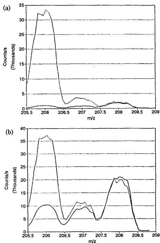
Fig. 5. Pb isotope peaks illustrating isotope dilution method (dotted line: 0.5 ml blood + 0.29 µg  $^{206}\text{Pb}$  solid line: no spiking) (a) level 1, (b) level 3.
