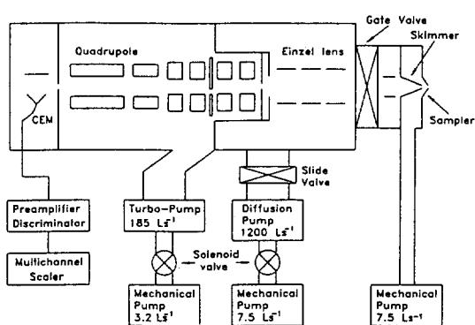
Fig. 1. Schematic diagram of ICP-MS system.
