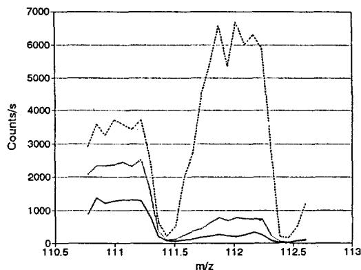
Fig. 6. Cd isotope peaks illustrating isotope dilution method (solid line: 0.5 ml level 1 blood + 5 ng  $^{111}\text{Cd}$ . Dotted line: 0.5 ml level 3 blood + 12 ng  $^{111}\text{Cd}$ . Centred line: 10 ppb Cd standard).
