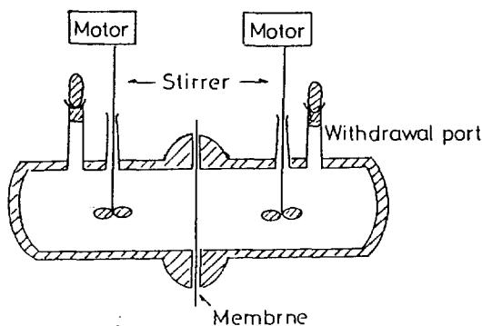
Fig. 1. The diffusion cell for measuring solute permeability.
