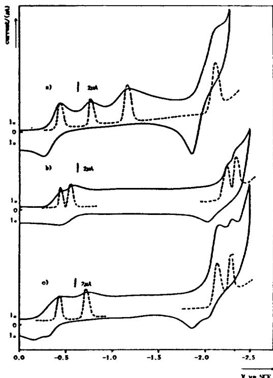
Fig. 6. Cyclic voltammogram (—) and differential pulse polarogram (---) of cobalt(II) complex (3a) in 0.1 M TEAP-Py(a), 0.1 M TEAP-DMSO(b) and 0.1 M TEAP-DMF(c) solution at scan rate was 50 mV/sec.
