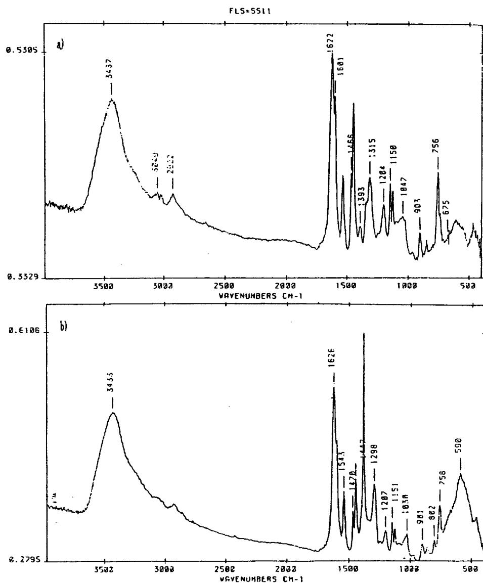
Fig. 1. Infrared absorption spectra of a) cobalt(II) (1a) and b) manganese(II) (1b) complexes.
