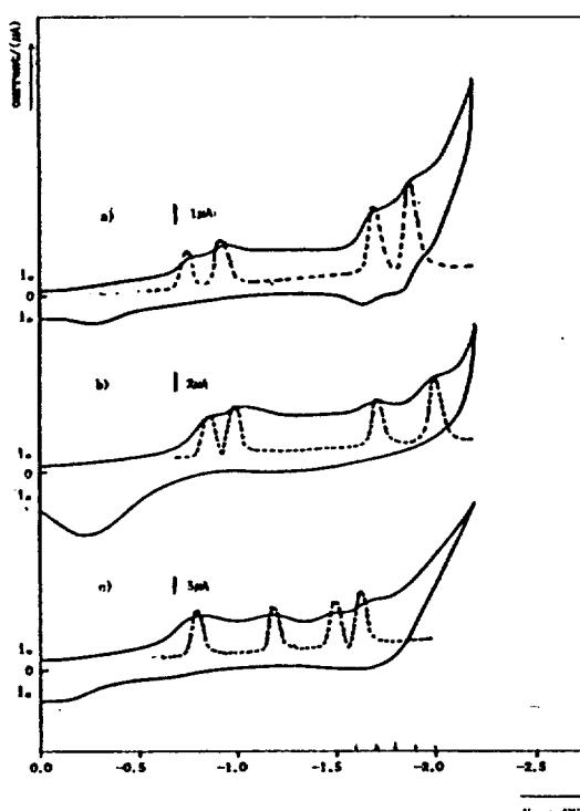
Fig. 5. Cyclic voltammogram (—) and differential pulse polarogram (---) of cobalt(II) complex (2a) in 0.1 M TEAP-Py(a), 0.1 M TEAP-DMSO(b) and 0.1 M TEAP-DMF(c) solution at scan rate was 50 mV/sec.
