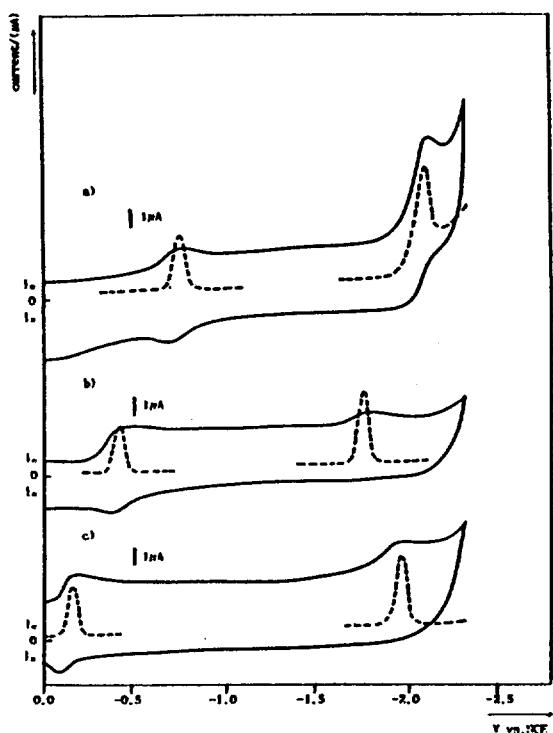
Fig. 4. Cyclic voltammogram (—) and differential pulse polarogram (---) of manganese(II) complex (1b) in 0.1 M TEAP-Py(a), 0.1 M TEAP-DMSO(b) and 0.1 M TEAP-DMF(c) solution at scan rate was 50 mV/sec.
