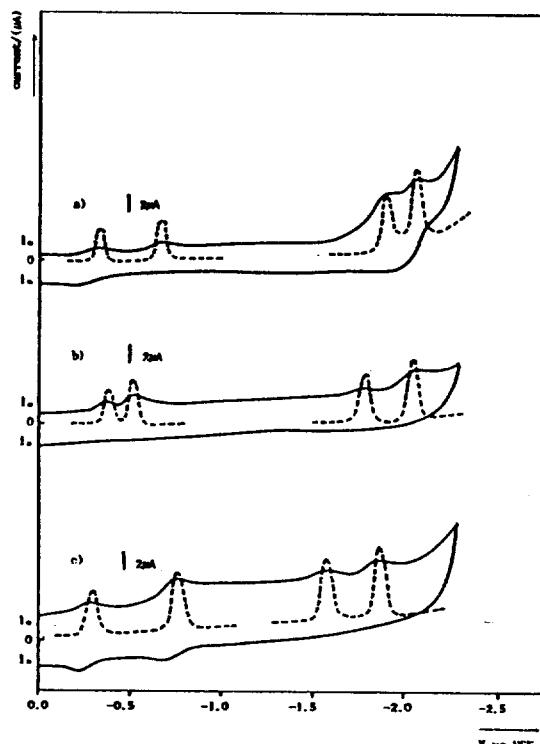
Fig. 7. Cyclic voltammogram (—) and differential pulse polarogram (---) of manganese(II) complex (2b) in 0.1 M TEAP-Py(a), 0.1 M TEAP-DMSO(b) and 0.1 M TEAP-DMF(c) solution at scan rate was 50 mV/sec.
