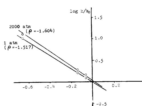
Fig. 2. The Hammett plots for the reaction of 2-phenethyl brosylate with substituted pyridines in acetonitrile at 50°C. The substituents included in this plot are the 4-NH<sub>2</sub>, 3,5-(CH<sub>3</sub>)<sub>2</sub>, 3-CH<sub>3</sub>, and H.
