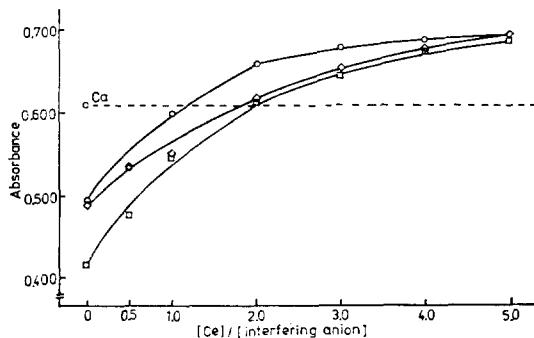
Fig. 10. Recovery of calcium ( $3.0 \times 10^{-4}$ M) absorption in the presence of interfering anions(ea.  $3.0 \times 10^{-4}$ M) by the addition of increasing amount of cerium in  $0.05\text{M}$  HCl solution. ○:  $\text{SO}_4^{2-}$ , □:  $\text{VO}_3^-$ , ◇:  $\text{SiO}_3^{2-}$ .
