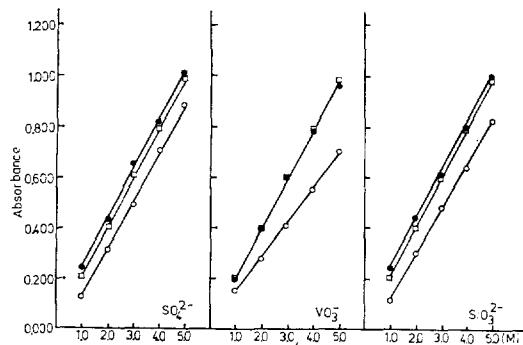
Fig. 11. Calibration curve for calcium showing the deviation from various interfering anions in  $0.05\text{M}$  HCl solution and the releasing effect of cerium. □: calcium only. ○: no cerium as the releasing agent. ●:  $6.0 \times 10^{-4}$  cerium as the releasing agent.
