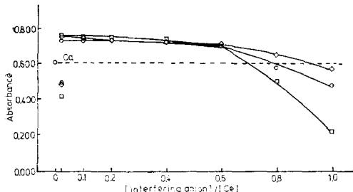
Fig. 12. The effect of various concentration in the interfering anions on the absorbance(0.610) of calcium ( $3.0 \times 10^{-4}$ M) in the presence of cerium( $1.5 \times 10^{-2}$ M) in 0.05M HCl solution. ○:  $\text{SO}_4^{2-}$ . □:  $\text{VO}_3^-$ . ◇:  $\text{SiO}_3^{2-}$ .
