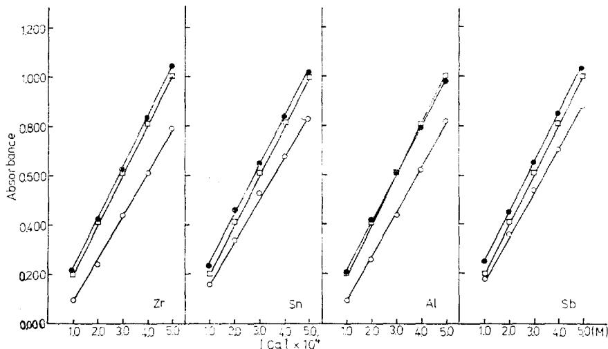
Fig. 5. Calibration curves for calcium showing the deviation by various interfering cations in 0.05M HCl solution. □: calcium only. ○: no cerium as the releasing agent. ●:  $6.0 \times 10^{-4}$ M cerium as the releasing agent.
