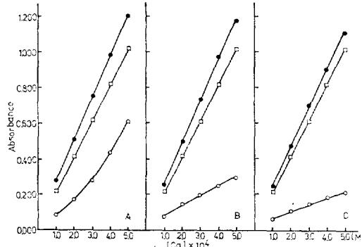
Fig. 13. Calibration curve for calcium showing the deviation from the concentration change of the mixed interfering anions ( $\text{SO}_4^{2-}$ ,  $\text{VO}_3^-$ ,  $\text{SiO}_3^{2-}$ ) in 0.05M HCl solution and the releasing effect of cerium. □: calcium only. ○: no cerium as the releasing agent. ●:  $1.5 \times 10^{-2}$ M cerium as the releasing agent. A: ea.  $3.0 \times 10^{-4}$ M. B: ea.  $1.5 \times 10^{-3}$ M. C: ea.  $3.0 \times 10^{-3}$ M.
