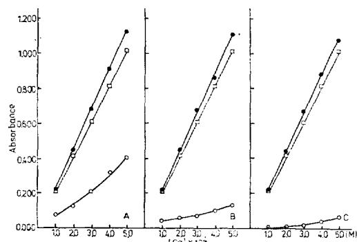
Fig. 14. Calibration curve for calcium showing the deviation from the concentration change of the mixed interfering cations and anions (Zr, Sn, Al, Sb,  $\text{SO}_4^{2-}$ ,  $\text{VO}_3^-$  and  $\text{SiO}_3^{2-}$ ) in 0.05M HCl solution and the releasing effect of cerium. □: calcium only. ○: no cerium as the releasing agent. ●:  $1.5 \times 10^{-2}$ M cerium as the releasing agent. A: ea.  $3.0 \times 10^{-4}$ M. B: ea.  $1.5 \times 10^{-3}$ M, C: ea.  $3.0 \times 10^{-3}$ M.
