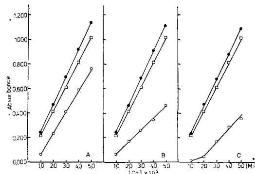
Fig. 8. Calibration curve for calcium showing the deviation from the concentration change of the mixed interfering cations(Zr, Sn, Al, Sb) in 0.05M HCl solution and the releasing effect of cerium. □: calcium only. ○: no cerium as the releasing agent. ●:  $1.5 \times 10^{-2}M$  cerium as the releasing agent. A: ea.  $3.0 \times 10^{-4}M$ . B: ea.  $1.5 \times 10^{-3}M$ . C: ea.  $3.0 \times 10^{-3}M$ .
