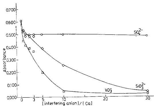
Fig. 9. The effect of various interfering anions on the absorbance (0.610) of calcium ( $3.0 \times 10^{-4}M$ ) in 0.05M HCl solution.
