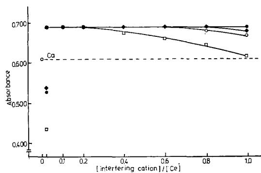
Fig. 7. The effect of various interfering cations on the absorbance (0.610) of calcium ( $3.0 \times 10^{-4}M$ ) in the presence of cerium ( $1.5 \times 10^{-2}M$ ) in 0.05M HCl solution. □:Zr. ●:Sn. ◆:Al. ○:Sb.
