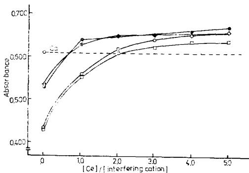
Fig. 4. Recovery of calcium ( $3.0 \times 10^{-4}$  M) absorption in the presence of interfering cations (ea.  $3.0 \times 10^{-4}$  M) by the addition of increasing amount of cerium in 0.05M HCl solution. ○:Zr. ●:Sn. □:Al. ◆:Sb.
