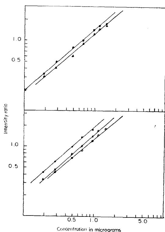
Fig. 3 Calibration Curves of Dy obtained from different carriers. ■ : KCl+LiF(1:1) △:LiF ● : AgCl+LiF(1:1) ▲ : KCl ○ : AgCl Step filter: 24.6% T Atmosphere control gas: Ar+O<sub>2</sub>(8:2)
