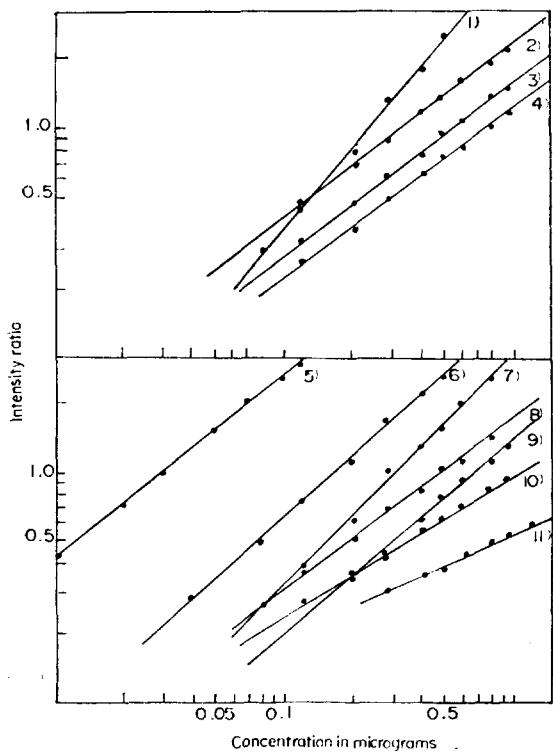
Fig. 5. Calibration curves of rare earth elements 1) Ho, 2) Gd, 3) Lu, 4) La, 5) Yb, 6) Dy, 7) Tm, 8) Eu, 9) Tb, 10) Er, 11) Sm. Carrier: KCl+LF. (1:1)/graphite powder (1:1) 10mig, Atmosphere control gas: Ar+O<sub>2</sub> (8:2), Step filter: 36.8% T.
