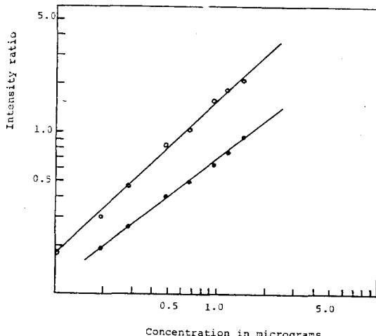
Fig. 2. Calibration Curves obtained from different analytical line. Carrier: KCl+LiF (1:1)/graphite powder(1:1), Atmosphere control gas: Ar+O<sub>2</sub>(8:2), Step filter: 24.6% T ○  $\frac{Er(3372.7 \text{ A})}{Y(3242.2 \text{ A})}$
