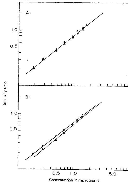
Fig. 4 Calibration curves of Er and Eu obtained from different atmosphere. ○ : Ar+O<sub>2</sub>(8:2) △ : Ar+O<sub>2</sub>(7:3) Carrier: KCl+LiF(1:1)/graphite powder(1:10mg), Step filter: 24.6% T, A:  $\frac{Eu(3971.9 \text{ Å})}{Y(3710.3 \text{ Å})}$
