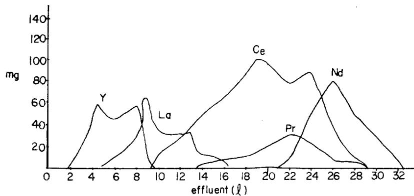
Fig. 2. Separation Curve of rare earth in monazite sand. Eluent; 0.0301 M EDTA; pH=8.4; column: 12.56 cm<sup>2</sup>×85 cm; resin: Dowex 1 (50~100 mesh); flow rate: 1 ml/min.
