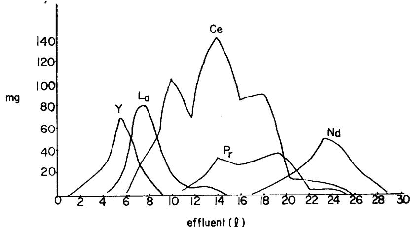
Fig. 1. Separation curve of rare earth in monazite sand. Eluent: 0.0301 M EDTA; pH=8.4; column: 19.63 cm<sup>2</sup>×65 cm; resin: Dowex 1 (50~100 mesh); flow rate: 1 ml/min.
