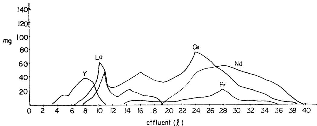
Fig. 3 Separation curve of rare earth in monazite sand. Eluent: 0.0301 M EDTA; pH=8.4; column: 12.56 cm<sup>2</sup>×85 cm; resin: Dowex 1 (50~100 mesh); flow rate: 2 ml/min.
