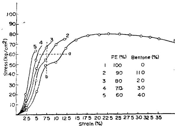
Fig. 2. Stress-strain curve.
