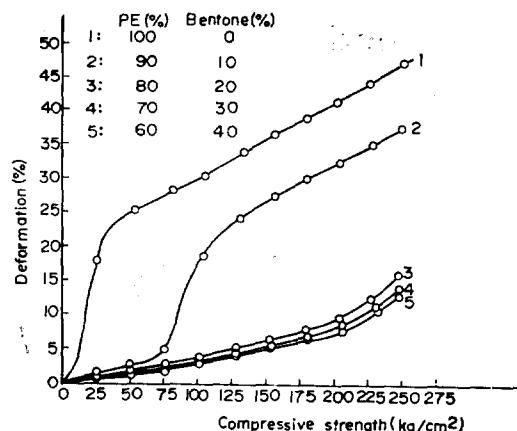
Fig. 3. Compressive strength of composites.
