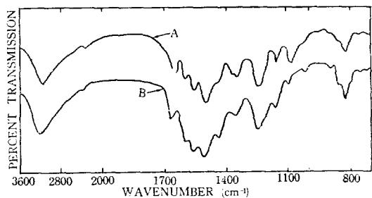
Figure 4. IR spectra of the oligomers
