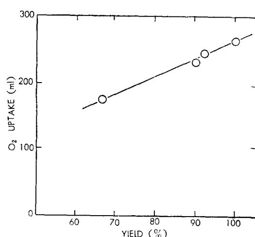
Figure 2. Linear relationship between the yield and O<sub>2</sub> uptake (pH 5~8)
