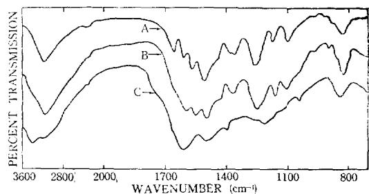
Figure 5. IR spectra of the heat-treated and untreated acetone soluble oligomers
