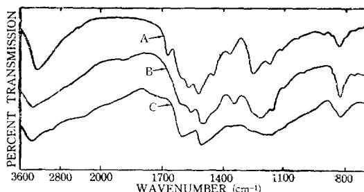
Figure 6. IR spectra of the heat-treated and untreated acetone insoluble oligomers
