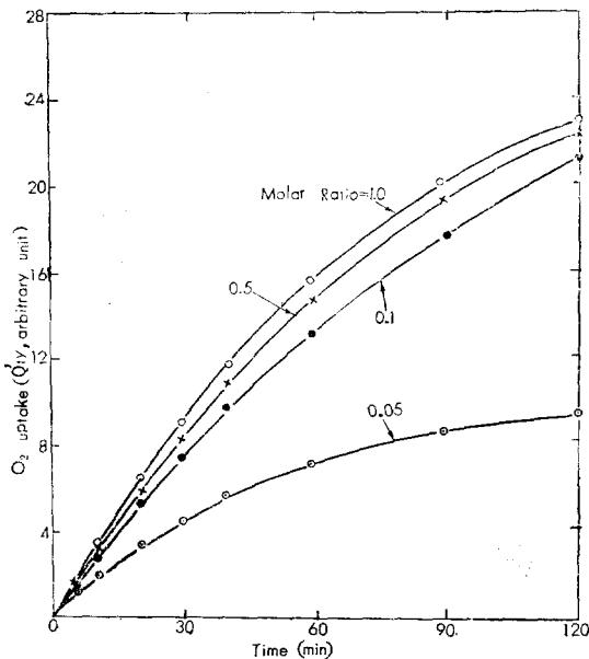
**Figure 3. Oxygen uptake plotted against time for different molar ratio (Fe-EDTA/*p*-aminophenol) at pH 8 ( $\text{NH}_4\text{Cl-NH}_4\text{OH}$  buffer) and 25°C**
