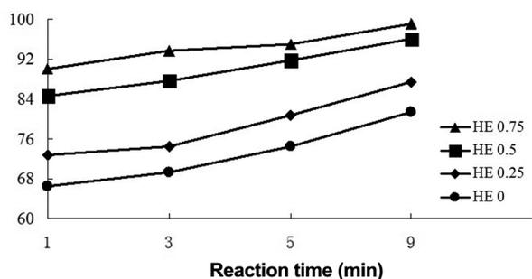
Figure 5. Effect of HE on WPO of oily wastewater. Conditions: temperature 340 °C, residence time 1 to 9 min, initial COD 18000 mg/L.
