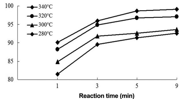
Figure 3. Effect of temperature on WPO of oily wastewater. Conditions: residence time 1 to 9 min, HE 0.75, initial COD 18000 mg/L.
