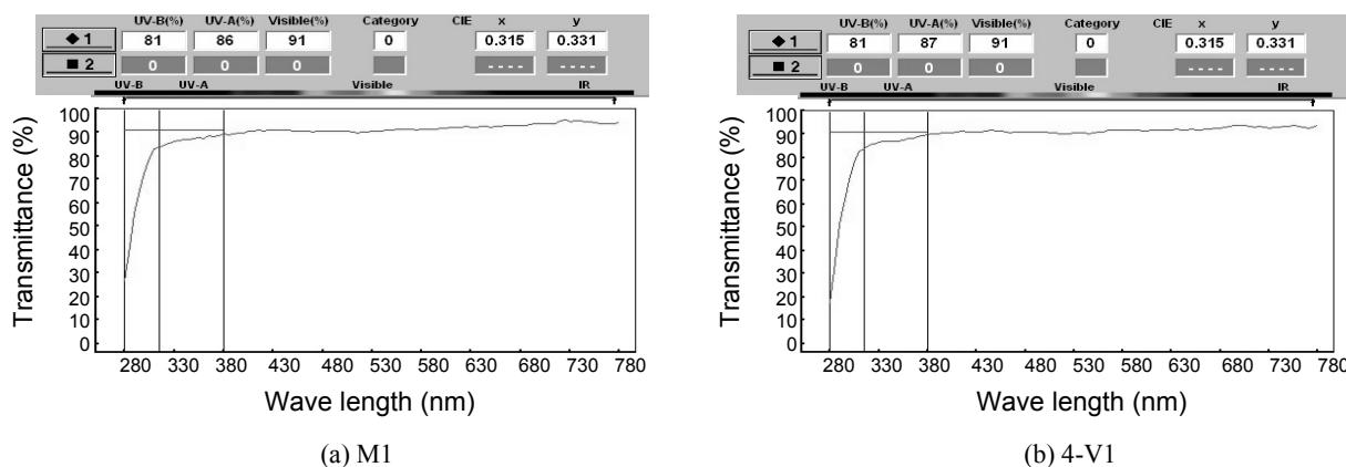
**Fig. 5.** Optical transmittance of M1 and 4-V1.
