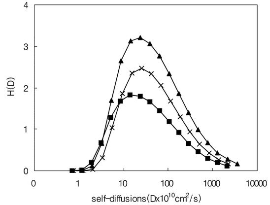
Fig. 4. Self-diffusion distributions of ester (■), PCL (▲), and PCL dyed type (×) polyurethane melts at 503 K.
