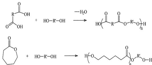
Scheme 1. Polymerization of ester and PCL type polyurethanes.
