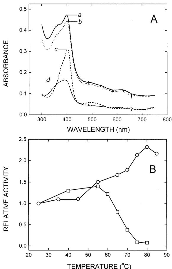
**Figure 2.** (A) Absorption spectra of HRP encapsulated in silica glass (*a, b*) and in aqueous solution (*c, d*) at 25 °C (*a, c*) and 80 °C (*b, d*). The HRP concentration was 5  $\mu\text{M}$  in 100 mM phosphate buffer (pH 7). Other conditions were the same as those in Figure 1A. (B) Catalytic activities of HRP in solution (*squares*) and encapsulated HRP (*circles*) as a function of temperature. The activity at 25 °C was set to 1.
