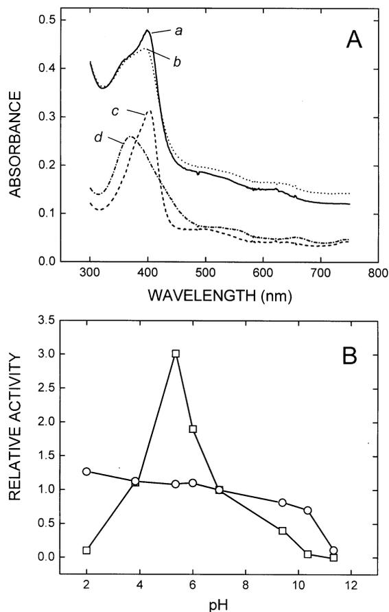
**Figure 1.** (A) Absorption spectra of HRP encapsulated in silica glass (*a, b*) and in aqueous solution (*c, d*) at pH 7 (*a, c*) and pH 2 (*b, d*). The spectra were obtained in a cuvette with 1 cm pathlength using a diode array spectrophotometer. The HRP concentration was 5  $\mu$ M in 100 mM phosphate buffer. (B) Catalytic activities of HRP in solution (*squares*) and encapsulated HRP (*circles*) as a function of pH. The activity at pH 7 was set to 1.
