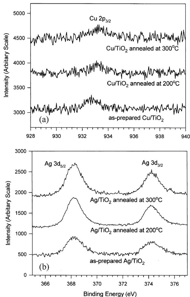
**Figure 5.** XPS spectra of Cu/TiO<sub>2</sub> and Ag/TiO<sub>2</sub> samples annealed at several temperatures (The concentration of Cu is 0.8 mole % and that of Ag is 1.5 mole %.); (a) Cu/TiO<sub>2</sub>; (b) Ag/TiO<sub>2</sub>.
