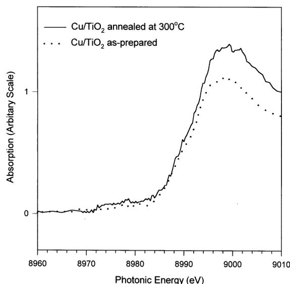
**Figure 6.** XANES spectra of Cu K-edge region for Cu/TiO<sub>2</sub> samples (The concentration of Cu is 0.8 mole %).
