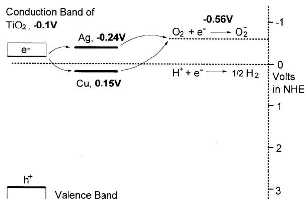
**Figure 2.** Schematic energy diagram of TiO<sub>2</sub>, loaded metals, and several electrolytes.
