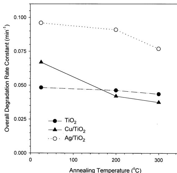
**Figure 3.** Photocatalytic activity of TiO<sub>2</sub>, Cu/TiO<sub>2</sub>, Ag/TiO<sub>2</sub> samples with the oxidation temperature (For Cu/TiO<sub>2</sub> the concentration of Cu is 0.8 mole %, and for Ag/TiO<sub>2</sub> that of Ag is 1.5 mole % relative to TiO<sub>2</sub>).
