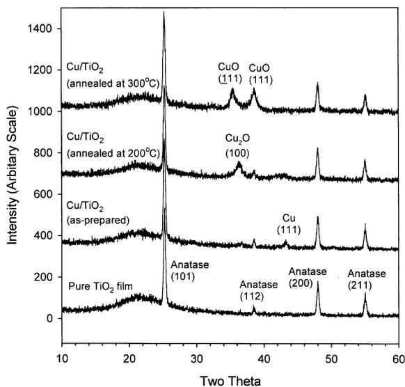
**Figure 4.** XRD patterns of Cu-loaded TiO<sub>2</sub> films annealed at several temperatures (TiO<sub>2</sub> film in anatase phase was deposited on a silica substrate at 450 °C with MOCVD method. Cu was deposited on TiO<sub>2</sub> film by photodecomposition method with 0.001 M CuSO<sub>4</sub> · 5H<sub>2</sub>O aqueous solution.).
