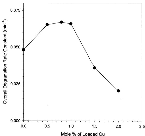
**Figure 1.** Photocatalytic activity of Cu/TiO<sub>2</sub> samples with the concentration of surface-loaded Cu (Model compound: DCB, 25 μM).
