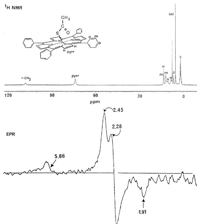
**Figure 2.** <sup>1</sup>H NMR (360 MHz) and EPR spectra for the reaction of ( $d_8$ -TPP)Fe(III)O<sub>3</sub>SCF<sub>3</sub> with 1.0 equiv. [CH<sub>3</sub>C(=O)S]<sup>-</sup>K<sup>+</sup>/methanol in dichloromethane solution. EPR spectrum was recorded at 77 K with 6000 G sweep, 9.19 GHz, 100 KHz modulation at 5 mwatt.
