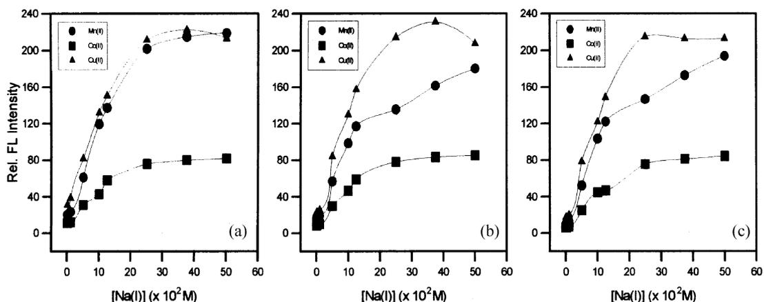
**Figure 6.** Enhanced fluorescence intensities in quenched anthrylazacrown ethers by Mn(II), Co(II) and Cu(II) with the concentration of added sodium nitrate; (a) Anthryl DA15C5, (b) Anthryl MA18C6, (c) Anthryl DA18C6. All solution were mixed with [anthrylazacrown ethers]= $1.0 \times 10^{-7}$  M and  $[M]=5.0 \times 10^{-4}$  M. (M=Mn(II), Co(II), Cu(II)). Excitation was at 254 nm and emission maximum centered near 412 nm.
