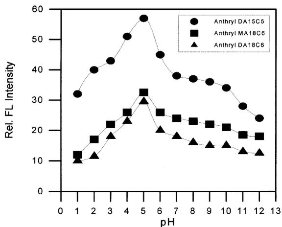
**Figure 3.** pH-fluorescence profiles for 0.1  $\mu\text{M}$  solutions of Anthrylazacrown ethers. Excitation was at 254 nm; Emission was measured at the emission maximum centered near 412 nm. pHs were maintained using the following solutions; 0.2 M HCl (pH 1 and 2), 0.2 M Sodium acetate (pH 3, 4, 5 and 6), 0.2 M Tris (pH 7, 8 and 9), 0.2 M  $\text{NaHCO}_3$  (pH 10 and 11), 0.2 M NaOH (pH 12).
