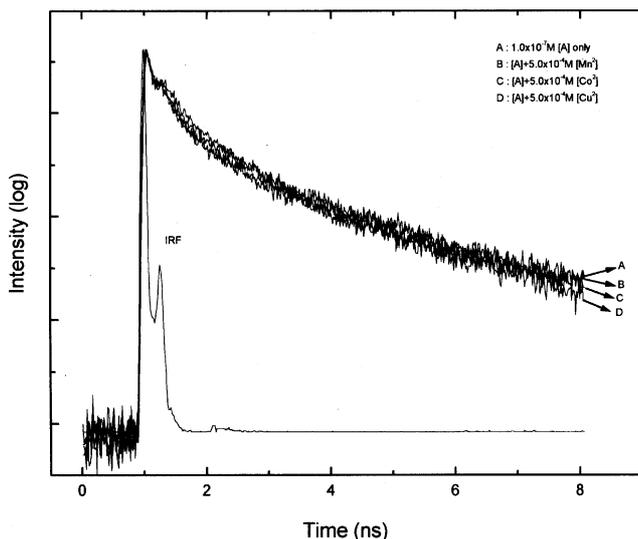
**Figure 5.** TCSPC spectrum of aqueous  $10^{-7}$  M of Anthryl DA15C5 at pH=5 without and with the metal ions  $Mn^{2+}$ ,  $Co^{2+}$ , and  $Cu^{2+}$ . The concentration of metal ion is  $5.0 \times 10^{-5}$  M. The excitation wavelength is 300 nm, and the detection wavelength is 410 nm. The notation IRF is the instrumental response function.
