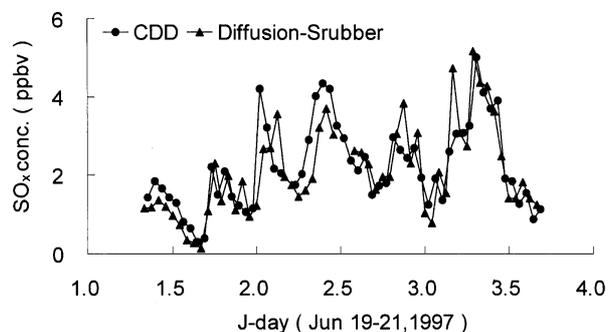
**Figure 4.** Temporal variation of  $\text{SO}_x$  gas in Seoul air monitored by CDD-IC and DS-IC method.
