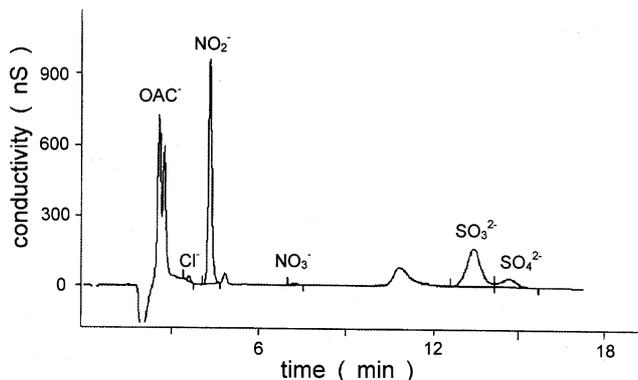
Figure 5. Typical ion chromatogram for Seoul air.
