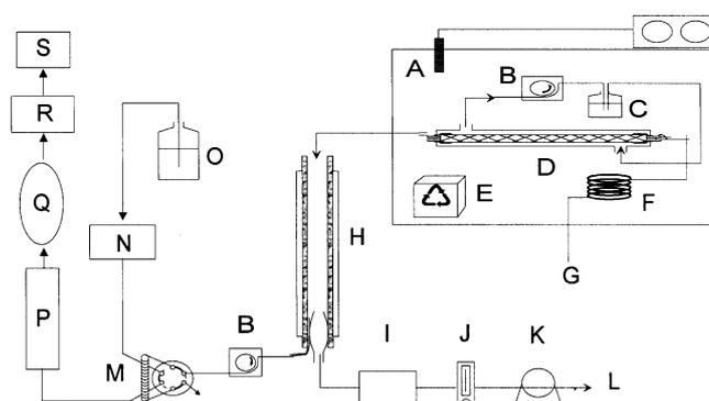
**Figure 1.** Schematic diagram of CDD/IC system. A: thermocouple, B: peristaltic pump, C: D. I. water, D: Nafion humidity controller, E: heater & fan, F: copper tubing, G: air inlet, H: CDD, I: pulse damper, J: flow meter, K: air pump, L: air outlet, M: injection valve, N: HPLC pump, O: eluent, P: IC column, Q: suppressor, R: detector, S: data analysis system
