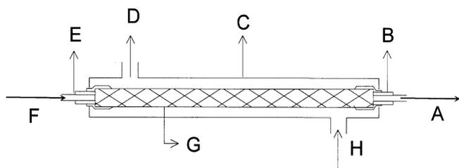
**Figure 2.** Schematic diagram of Nafion humidity controller. A: air outlet, B: tygon tubing, C: glass tubing, D: D. I. water outlet, E: PE tubing, F: air inlet, G: Nafion tubing, H: D. I. water inlet
