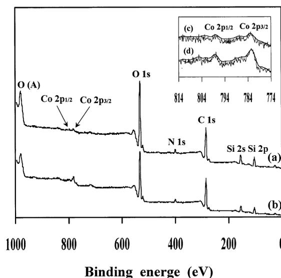
**Figure 8.** X-ray photoelectron spectra of (a) Co/APTMS/MCM-41 and (b) Co/AAPTMS/MCM-41. Inset shows the smoothed and enlarged XP spectra of the cobalt 2p photoelectron region of (c) spectrum (a) and (d) spectrum (b).
