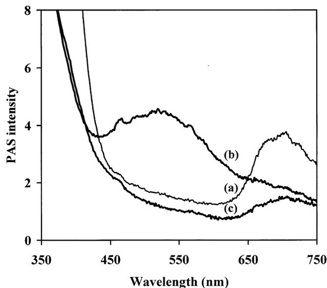
**Figure 6.** Photoacoustic spectra of (a) calcined MCM-41, (b) APTMS/MCM-41, and (c) AAPTMS/MCM-41 treated at room temperature for 1 h with Reichardt's dye solution (10 mL,  $10^{-4}$  M), respectively.
