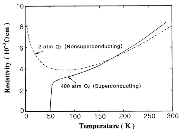
**Figure 5.** Electrical resistivity vs temperature for superconducting and non-superconducting  $\text{La}_{1.82}\text{Ca}_{1.18}\text{Cu}_2\text{O}_6$ .
