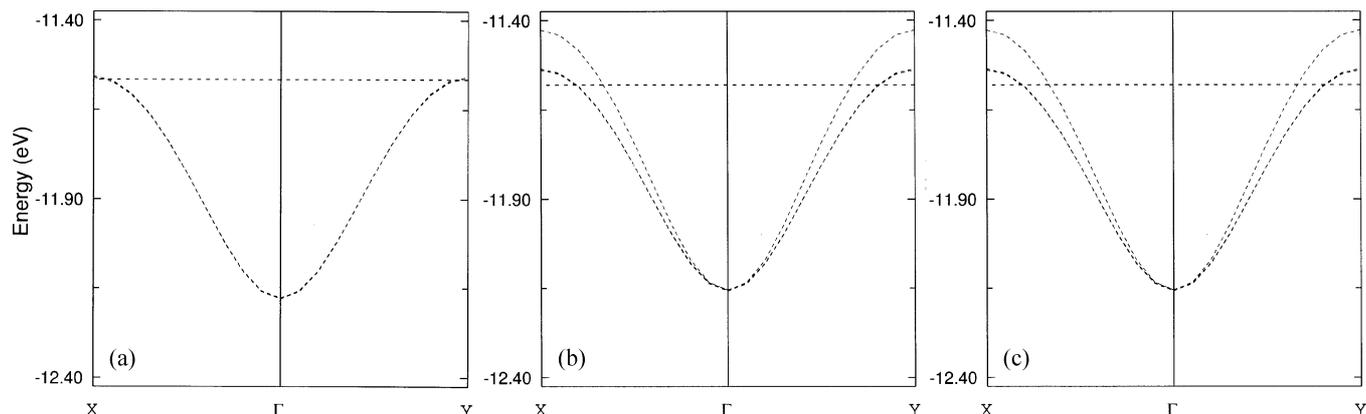
**Figure 3.** The band dispersion near the Fermi energy obtained from the structure of (a) the non-superconducting 2126 phase, (b) the superconducting 2126 phase with one additional oxygen, and (c) the superconducting phase with two additional oxygen atoms in a unit cell at room temperature.
