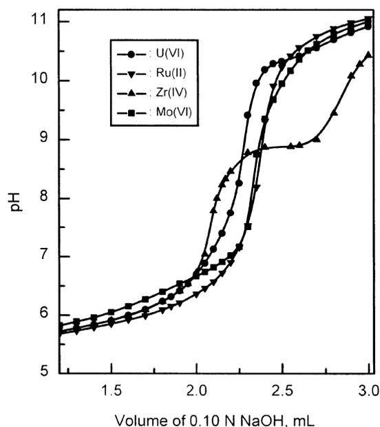
**Figure 2.** Alkalimetric titration curves for  $\text{HNO}_3$ -metal ion in 0.20 M potassium oxalate complexing medium;  $\text{HNO}_3$ : 0.202 meq, metal ion: 0.02 mmole.
