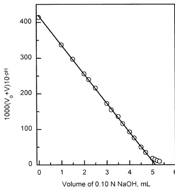
**Figure 7.** Gran plot for the alkalimetric titration of free acid in a simulated spent fuel solution by the noncomplexing method; HNO<sub>3</sub>: 0.5034 meq, U: 50 mg, Cs: 125  $\mu$ g, Ce: 125  $\mu$ g, Mo: 176  $\mu$ g, Nd: 213  $\mu$ g, Ru: 117  $\mu$ g, Zr: 190  $\mu$ g.
