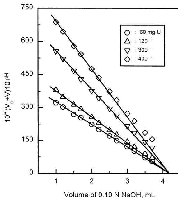
**Figure 5.** Effect of uranium concentration on Gran plot for the alkalimetric titration of free acid in the 0.20 M potassium oxalate medium; HNO<sub>3</sub>: 0.4126 meq.
