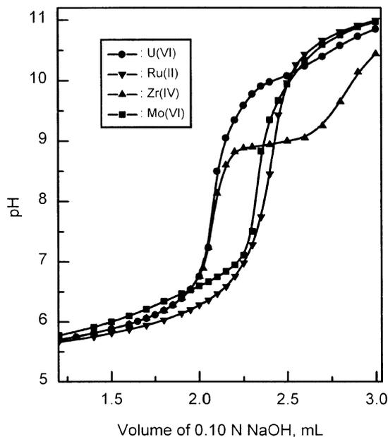
**Figure 3.** Alkalimetric titration curves for  $\text{HNO}_3$ -metal ion in mixed 0.10 M potassium oxalate-0.10 M potassium fluoride complexing medium;  $\text{HNO}_3$ : 0.202 meq, metal ion: 0.02 mmole.
