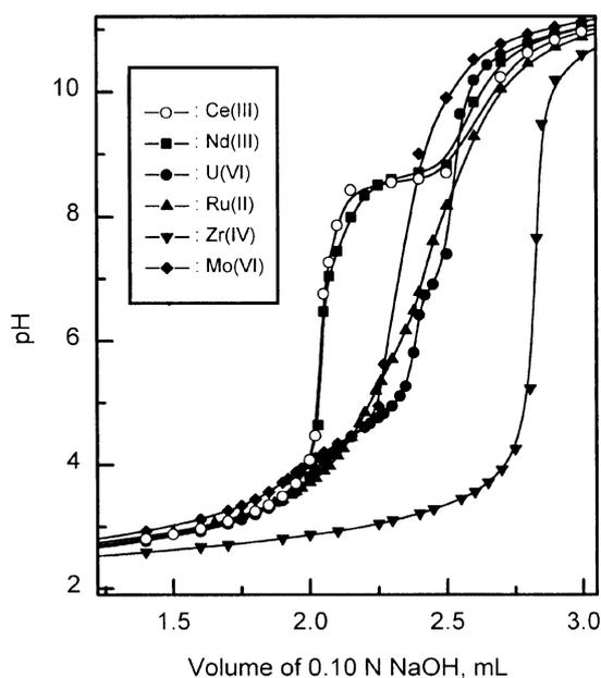
**Figure 1.** Alkalimetric titration curves for HNO<sub>3</sub>-metal ion in noncomplexing medium; HNO<sub>3</sub>: 0.202 meq, metal ion: 0.02 mmole.
