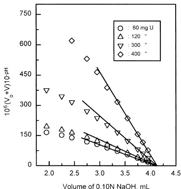
**Figure 6.** Effect of uranium concentration on Gran plot for the alkalimetric titration of free acid in the mixed 0.10 M potassium oxalate-0.10 M potassium fluoride medium; HNO<sub>3</sub>: 0.4126 meq.
