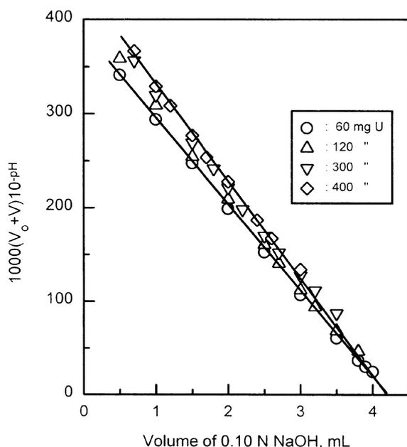
**Figure 4.** Effect of uranium concentration on Gran plot for the alkalimetric titration of free acid in noncomplexing medium; HNO<sub>3</sub>: 0.4126 meq.
