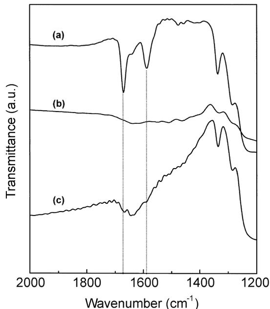
**Figure 2.** FT-IR spectra of 2-EAQ/Pd-Y after (a) evacuation at 200 °C for 2 h, (b) adsorption of 10 torr of H<sub>2</sub> at RT for 20 min., and (c) adsorption of 10 torr of O<sub>2</sub> at RT for 20 min.
