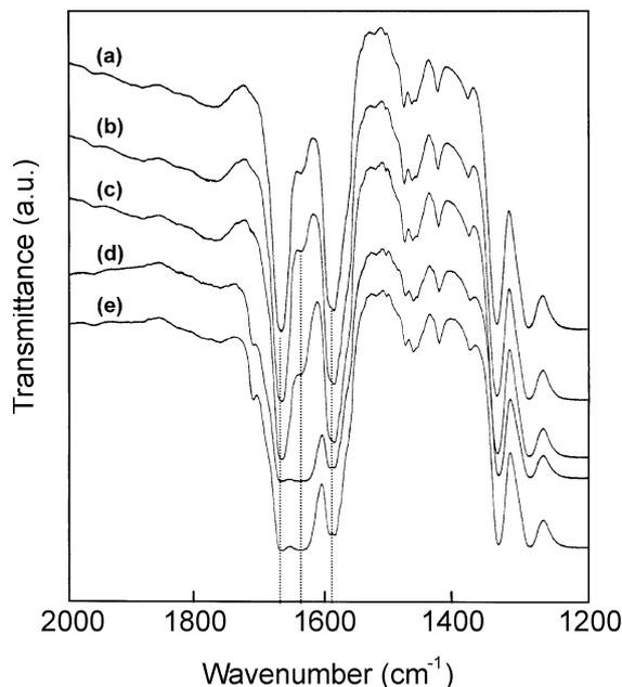
**Figure 1.** FT-IR spectra of 2-EAQ-Y after (a) evacuation at 200 °C for 2 h, (b) adsorption of 10 torr of H<sub>2</sub> at RT for 20 min, (c) adsorption of 10 torr of O<sub>2</sub> at RT for 20 min., (d) heating at 60 °C for 10 min., and (e) evacuation at room temperature.
