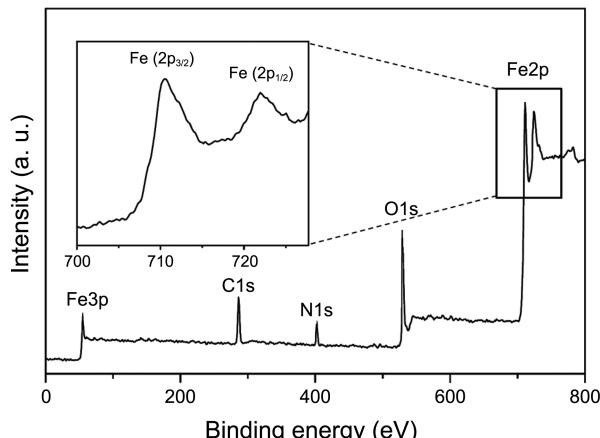
**Figure 1.** Survey scan of gelatin- $\text{Fe}_3\text{O}_4$  composite and its high-resolution XPS spectrum of  $\text{Fe}2\text{p}$ .
