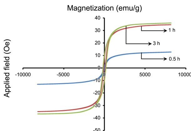
**Figure 8.** VSM curves of synthesized  $\gamma$ -Fe<sub>2</sub>O<sub>3</sub> nanoparticles at 600 °C in different times of curing in furnace.
