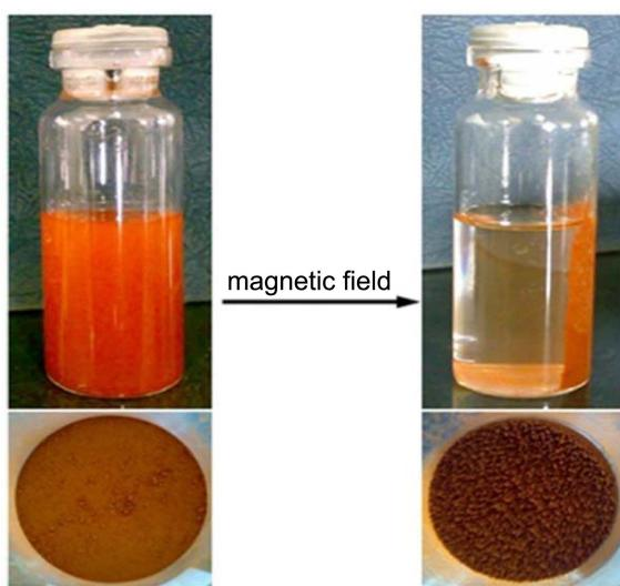
**Figure 3.** The produced maghemite nanoparticles dispersed in ethanol at absence and present of magnetic field.
