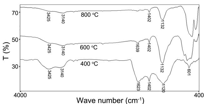
**Figure 4.** FT-IR spectra of gelatin-Fe<sub>3</sub>O<sub>4</sub> nanocomposite at 400 °C,  $\gamma$ -Fe<sub>2</sub>O<sub>3</sub> nanoparticles at 600 °C and  $\alpha$ -Fe<sub>2</sub>O<sub>3</sub> nanoparticles at 800 °C.
