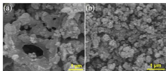
**Figure 5.** SEM images of (a) gelatin-Fe<sub>3</sub>O<sub>4</sub> nanocomposite after 1 h curing at 500 °C and (b) synthesized  $\gamma$ -Fe<sub>2</sub>O<sub>3</sub> nanoparticles after 1 h curing at 600 °C (complete decomposition of gelatin).
