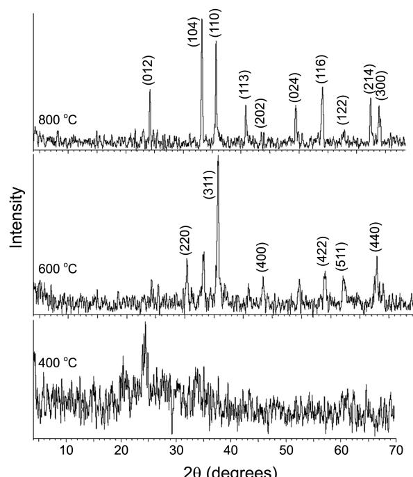
**Figure 2.** XRD patterns of gelatin- $\text{Fe}_3\text{O}_4$  nanocomposite at 400 °C,  $\gamma\text{-Fe}_2\text{O}_3$  nanoparticles at 600 °C.
