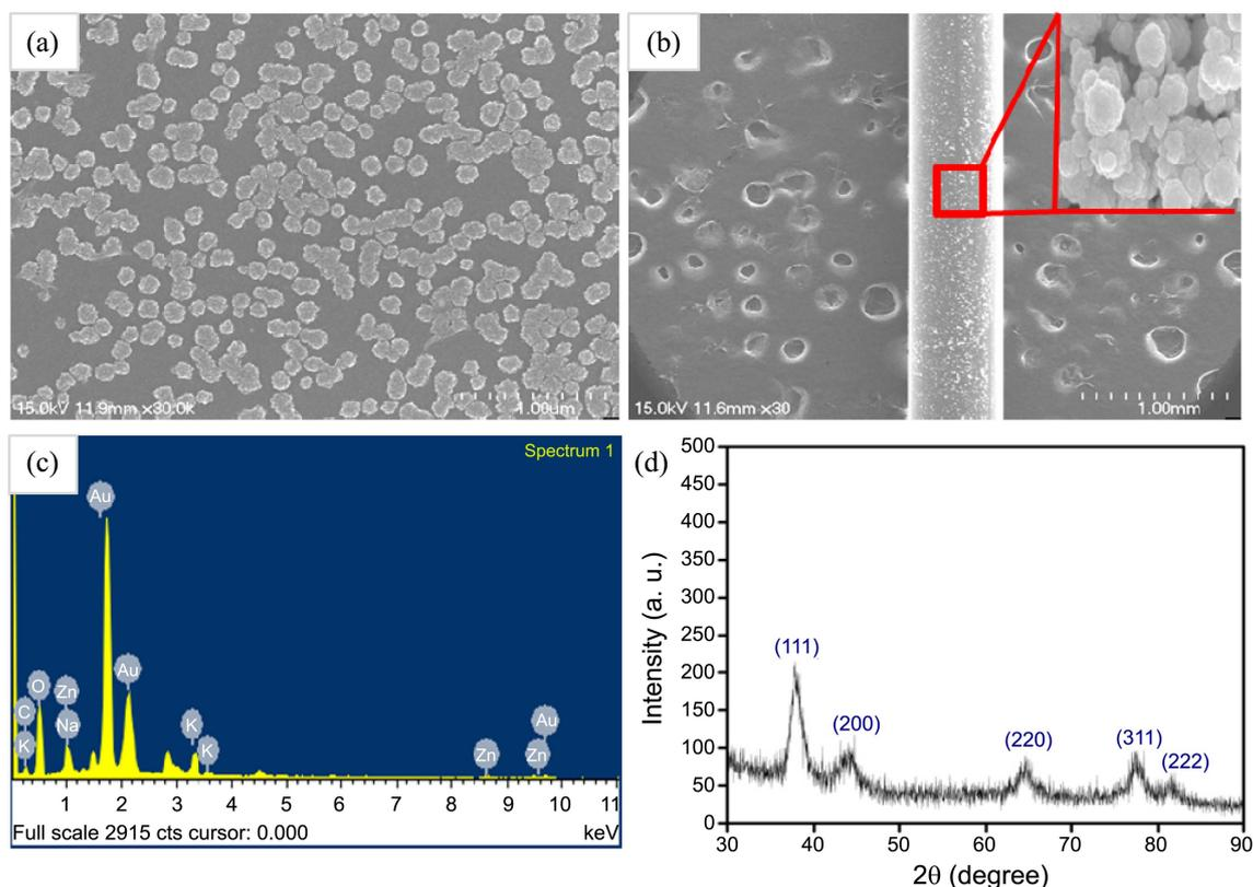
**Figure 2.** SEM images of (a) chitosan nanoparticles, (b) chitosan-gold nanocomposites on the optical fiber, (c) EDX analysis of chitosan-gold nanocomposites on optical fiber, (d) XRD analysis of chitosan-gold nanocomposites on the SiO<sub>2</sub> substrates.
