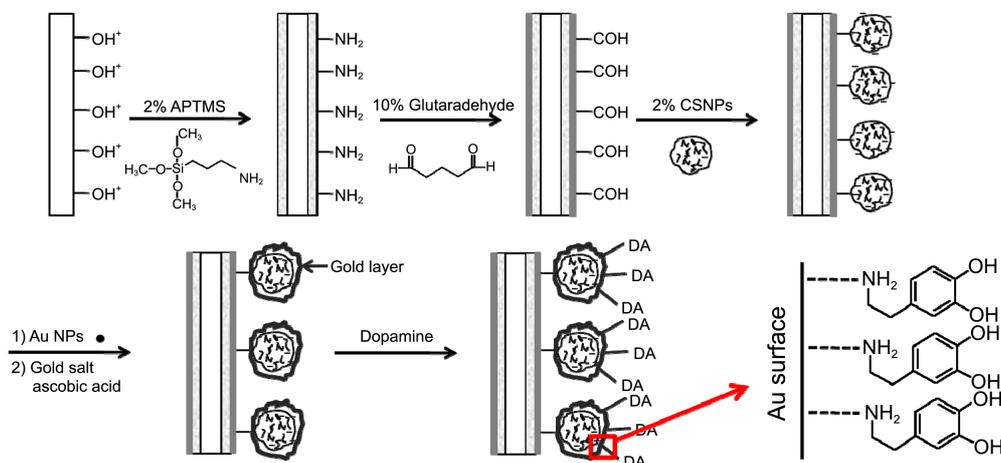
**Scheme 1.** Schematic fabrication steps to prepare chitosan-gold nanocomposites arrayed on optical fiber for Raman measurements of dopamine molecules.
