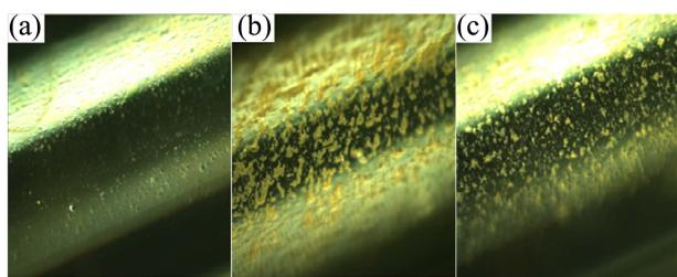
**Figure 4.** Microscopy images of (a) a optical fiber, (b) Chitosan-gold nanocomposites on the optical fiber, and (c) dopamine adsorbed chitosan-gold nanocomposites on the optical fiber.
