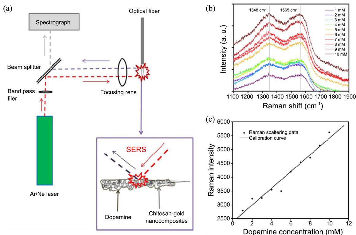
**Figure 5.** (a) Schematic diagram of SERS measurement system, (b) Raman spectra of dopamine molecules adsorbed on chitosan-gold nanocomposites on the optical fiber over dopamine concentration ranges, (c) Calibration curve of Raman intensity at  $1348\text{ cm}^{-1}$  vs. dopamine concentration ranges (1-10 mM).
