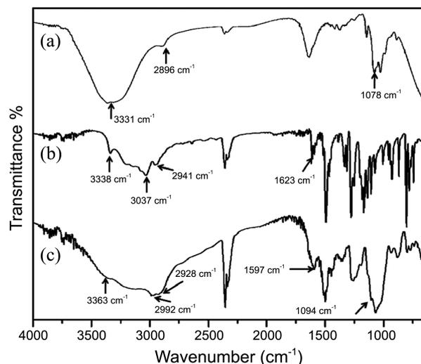
**Figure 3.** FT-IR spectra of (a) chitosan-gold nanocomposites, (b) Dopamine, (c) dopamine-adsorbed chitosan-gold nanocomposites.
