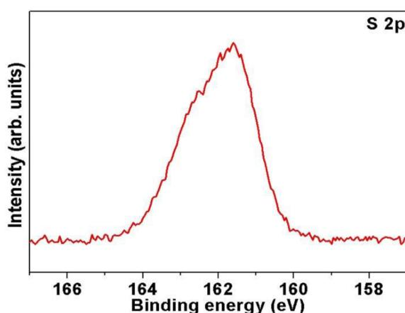
**Figure S1.** S 2p XPS spectrum of thiolated CNTs. An asymmetric peak is detected at 162 eV due to the S 2p photoelectron signal from the thiolate bond.<sup>1,2</sup>
