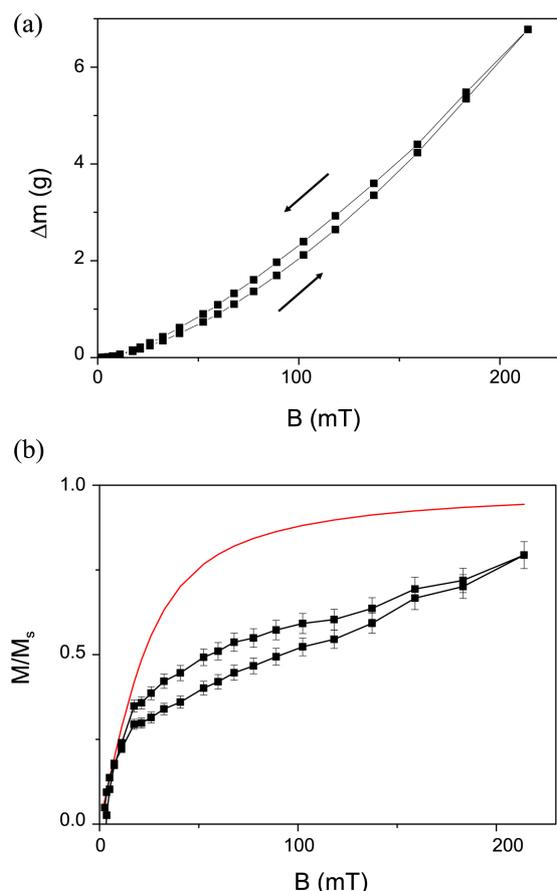
**Figure 2.** (a) Magnetic weight of the 3 wt % sample at different magnetic fields. As the magnetic weight changes slowly following an instantaneous shift at high fields, it is measured at 5 min after the magnetic field is set. (b) Magnetization of the sample calculated from Eq. (1), the magnetic weights of Figure 2(a) and the magnetic field gradient of Figure 1(b). The curve above the magnetization data represents the Langevin function.
