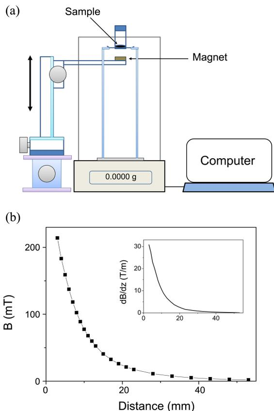
**Figure 1.** (a) Magnetic weight by magnetization of the sample is measured with an electronic balance connected to a computer. (b) Magnetic field strength measured at different positions between the sample and the magnet. Inset shows the magnetic field gradient evaluated from the measured magnetic field.
