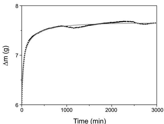
**Figure 3.** Temporal change of magnetic weight of the 3 wt % sample when the sample is placed at magnetic field of 212 mT. Fitting curve of the stretched exponential function of Eq. (3) is overlapped and the analysis results are given in Table 1.
