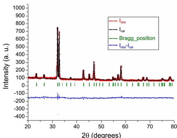
**Figure 2.** Rietveld refinement profile for the fit to the XRD pattern of  $\text{LaSr}_2\text{MnCrO}_7$ .
