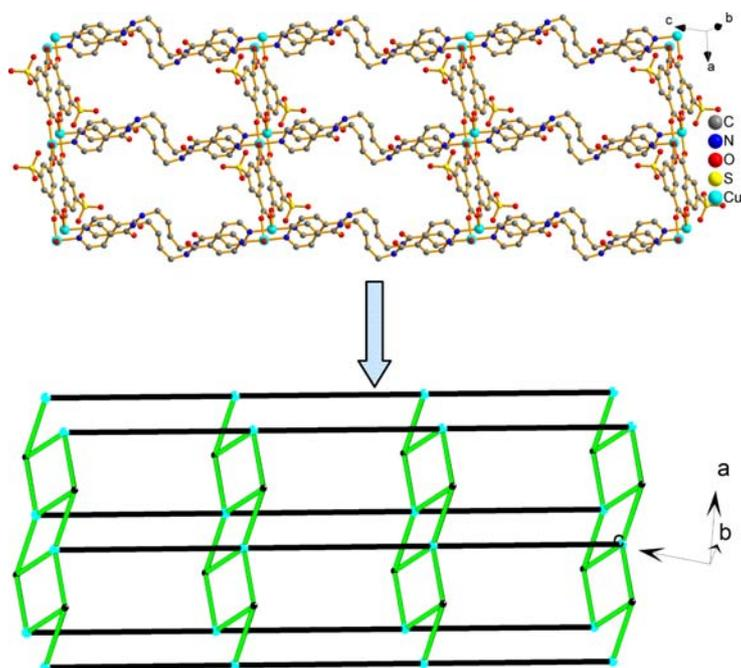
**Fig S3.** The ball-and-stick model of 2D double-layer in compound **1** (top). The schematic view of this 2D double-layer (bottom).
