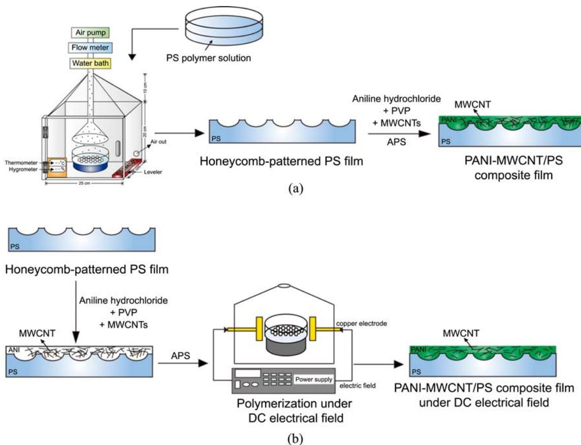
**Figure 1.** (a) Overall scheme for the formation of the PANI thin layer on the honeycomb-patterned PS film for the PANI-MWCNT/PS composite film, (b) the system for the formation of honeycomb-patterned PANI-MWCNT/PS composite film under DC electrical field.
