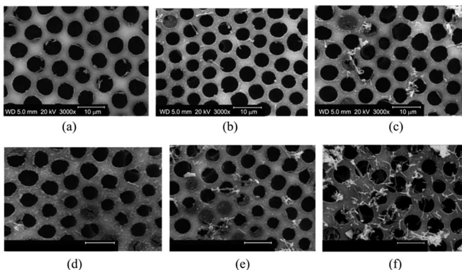
**Figure 4.** SEM images showing the formation of the PANI-MWCNT/PS composite film. The images of (a), (b), and (c) show the typical SEM images with the degree of adsorption of MWCNTs in the PANI/PS film at polymerization times of 1, 2, and 8 h, respectively when 1% (wt % to aniline) of MWCNT was dispersed in the aniline solution. The images of (d), (e), and (f) show the SEM images obtained using 3 wt % of MWCNT under same polymerization time.
