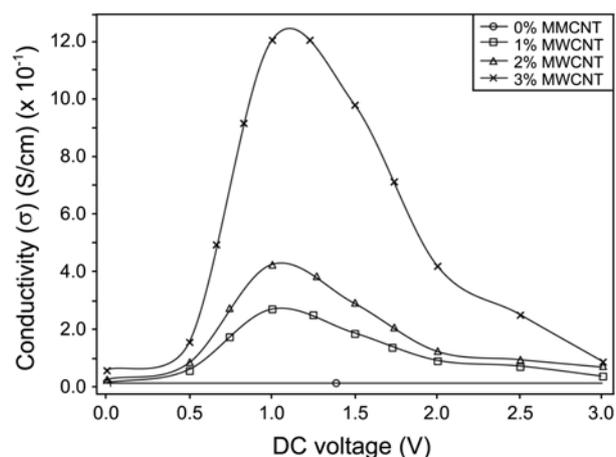
**Figure 9.** Room temperature DC conductivity depending on the loaded electrical field.
