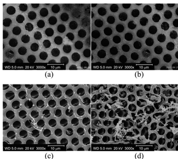
**Figure 7.** Typical SEM images showing the effect of loaded electrical field on the the formation of the PANI-MWCNT/PS composite film obtained by the loaded voltage of 3.0 V. (a), (b), (c), and (d) show the SEM images of PANI-MWCNT/PS composite with the polymerization time of 1, 2, 6, and 8 h, respectively.
