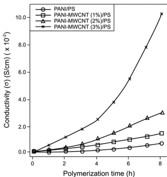
**Figure 5.** Room temperature DC conductivity depending on the time of polymerization and added MWCNT concentration (wt %).
