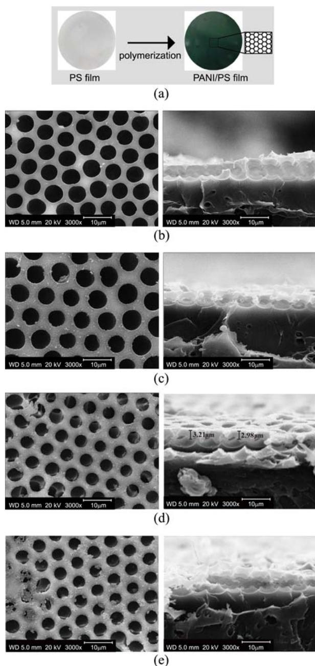
**Figure 3.** SEM images showing the formation of the PANI thin layer on the surface of the patterned PS film. (a) Color change from transparent to green at 2 h polymerization of aniline on the surface of the PS film. The images of (b), (c), (d), and (e) show the effect of polymerization time for the formation of the PANI thin layer on the surface of the patterned PS film by increasing the polymerization time with 1, 2, 6, and 8 h, respectively.
