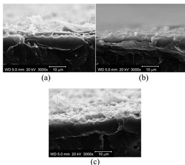
**Figure 8.** Cross sectional SEM images showing the effect of loaded electrical field on formation of the PANI-MWCNT/PS composite film. (a), (b), and (c) show the images obtained at the loaded voltage of 0 V, 1.0 V, and 3.0 V, respectively. For the PANI-MWCNT thin layer, 3 wt% MWCNT was used with 6 h polymerization.
