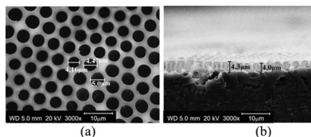
**Figure 2.** Typical SEM images of the honeycomb-patterned PS film used as a template for the PANI/PS film. (a) Surface image, (b) cross sectional image.
