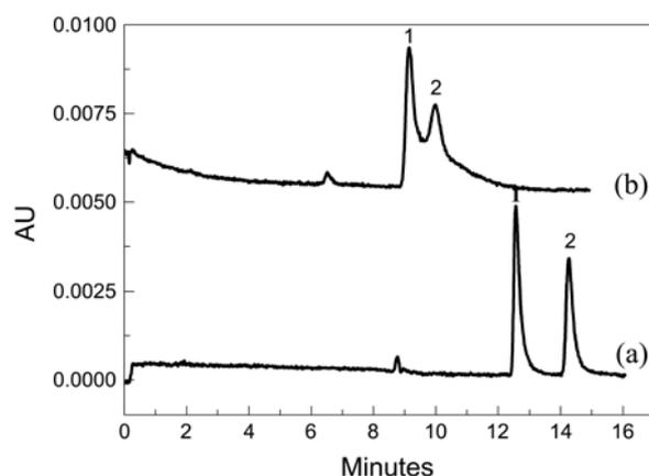
**Figure 4.** Electrochromatograms of carbendazim and imidacloprid obtained on LCCE-TMOS-VTMS column (a) and TMOS-VTMS column (b). Mobile phase, 20 mmol·L<sup>-1</sup> phosphate buffer (pH 7.0) - acetonitrile (90: 10, v/v). Other conditions are the same as in Fig. 3. Peak identification: 1, carbendazim; 2, imidacloprid.
