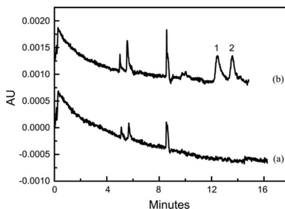
**Figure 6.** Electrochromatograms of carbendazim and imidacloprid in non-spiked tomato samples (a) and spiked tomato samples (b). Mobile phase, 20 mmol·L<sup>-1</sup> phosphate buffer (pH 7.0)-acetonitrile (90:10, v/v). Other conditions are the same as in Fig. 3. Peak identification: 1, carbendazim; 2, imidacloprid.
