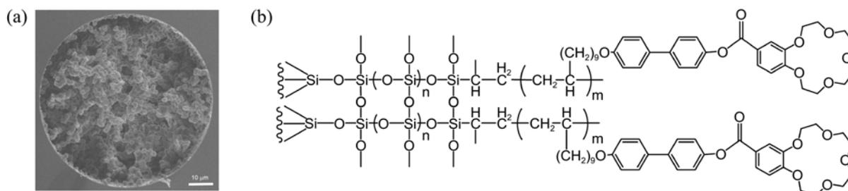
**Figure 1.** The scanning electron microscope image (a) and schematic (b) of LCCE-TMOS-VTMS column.
