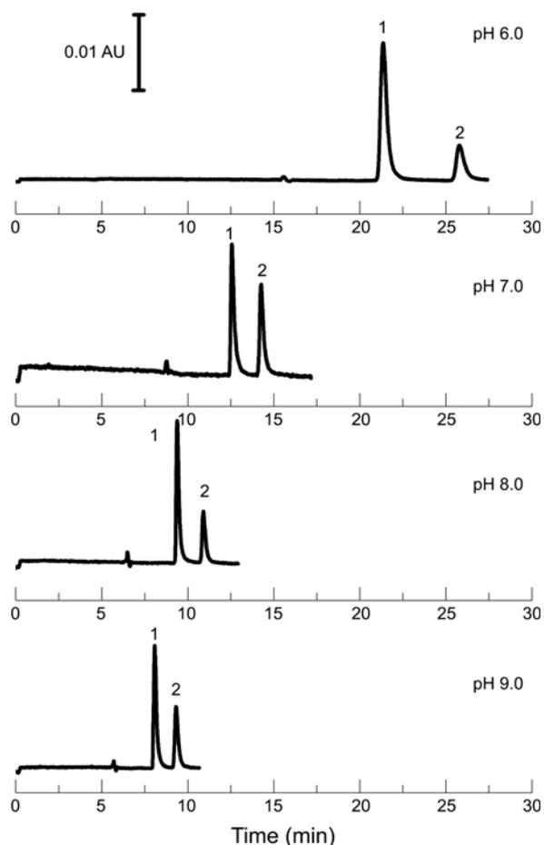
**Figure 3.** Effect of pH of running buffer on resolution. Mobile phase, 20 mmol·L<sup>-1</sup> phosphate buffer-acetonitrile (90:10, v/v); detection wavelength, 270 nm; applied voltage, 15 kV. Peak identification: 1, carbendazim; 2, imidacloprid.
