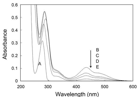
**Figure 1.** UV-vis absorption spectra of 91  $\mu\text{M}$  catechin: (a) in deaerated water, (b) in deaerated buffer solution at pH = 10.52, (c) in deaerated buffer solution at pH = 10.01, (d) in deaerated buffer solution at pH = 8.81, and (e) in aerated water.
