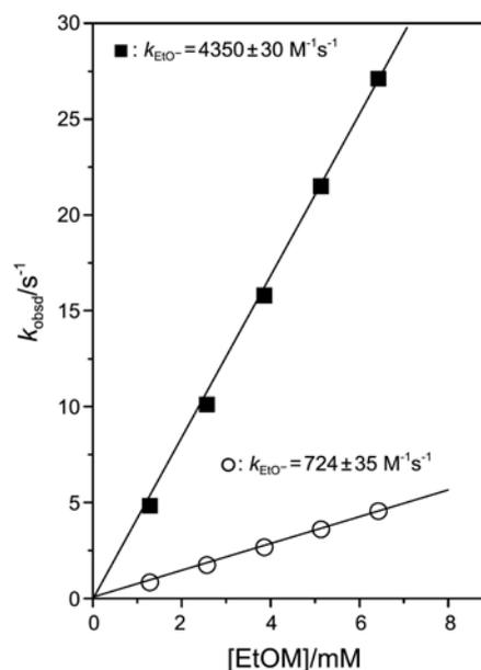
**Figure 4.** Plots of  $k_{\text{obsd}}$  vs.  $[\text{EtOK}]$  for reactions of 4-nitrophenyl nicotinate **5** (○) and isonicotinate **6** (■) with EtOK in the presence of 18C6 in anhydrous EtOH at  $25.0 \pm 0.1$  °C.  $[\text{18C6}]/[\text{EtOK}] = 2.0$ .
