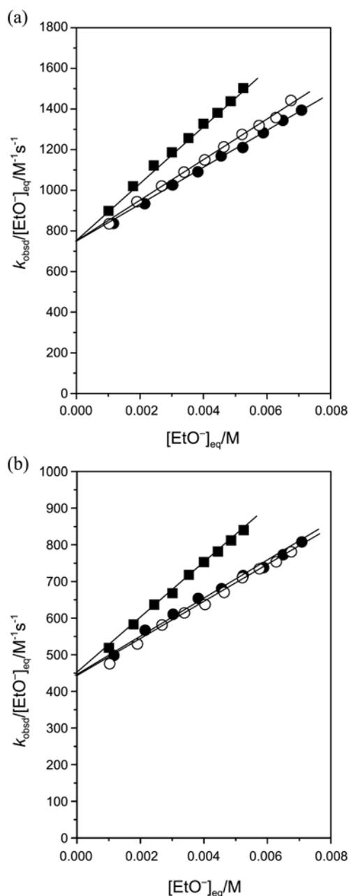
**Figure 3.** Plots of  $k_{\text{obsd}}/[\text{EtO}^-]_{\text{eq}}$  vs.  $[\text{EtO}^-]_{\text{eq}}$  for reactions of 4-nitrophenyl nicotinate **5** (a) and isonicotinate **6** (b) with EtOK (●), EtONa (○), and EtOLi (■) in anhydrous EtOH at  $25.0 \pm 0.1$  °C.
