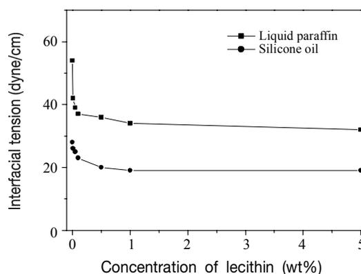
**Figure 2.** Interfacial tension between surfactants solution and liquid paraffin, silicone oil measured by ring method.
