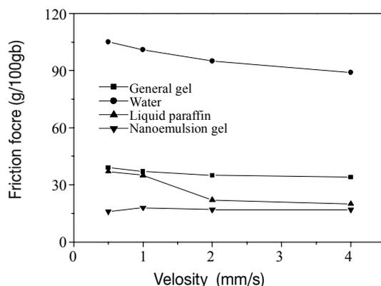
**Figure 6.** Results of friction test for nanoemulsion gel and general gel.
