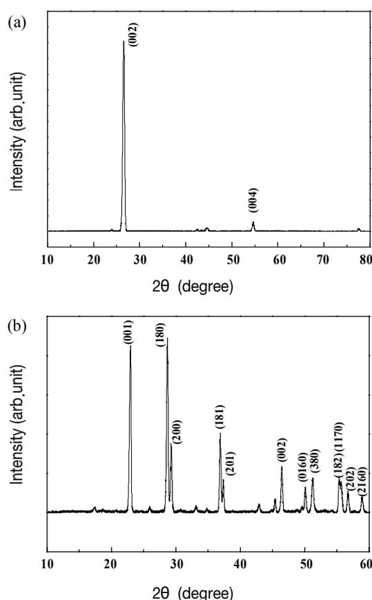
**Figure 1.** XRD patterns of (a) KS6 and (b) Nb<sub>2</sub>O<sub>5</sub>.
