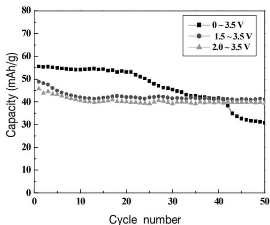
**Figure 3.** Specific discharge capacity vs. cycle number for the KS6/1.0 M LiPF<sub>6</sub>-EC:DEC(1:2)/Nb<sub>2</sub>O<sub>5</sub> system at a current density of 100 mA g<sup>-1</sup>.
