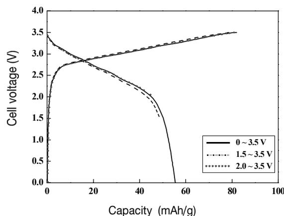
**Figure 2.** The initial charge/discharge curves for the KS6/1.0 M LiPF<sub>6</sub>-EC:DEC (1:2)/Nb<sub>2</sub>O<sub>5</sub> with an electrode mass ratio of 1:1.
