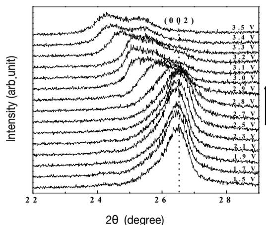
**Figure 4.** *In-situ* XRD patterns of the KS6 (graphite) electrode during the first charging process of the KS6/Nb<sub>2</sub>O<sub>5</sub> energy storage system for KS6 to Nb<sub>2</sub>O<sub>5</sub>.
