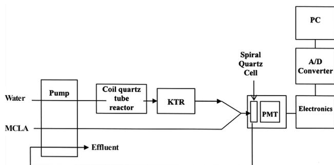
**Figure 1.** Schematic of the apparatus for investigating the mobility of  $\text{HO}_2\cdot/\text{O}_2^{\cdot-}$  molecules generated from the surface of illuminated  $\text{TiO}_2$  particles. KTR: knotted tube reactor; PMT: photomultiplier tube; A/D converter: analog-to-digital converter.
