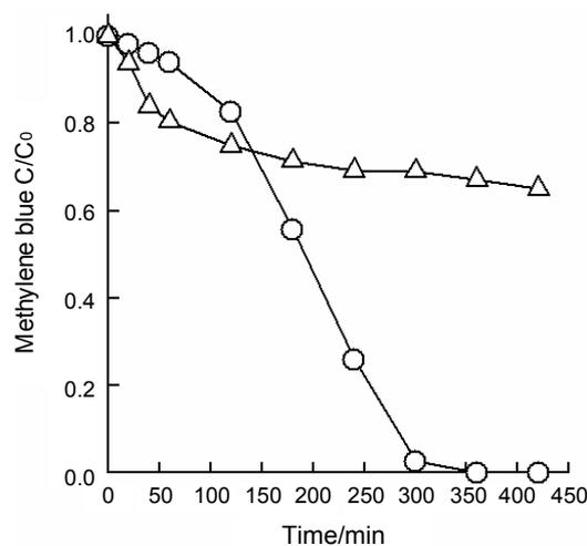
**Figure 8.** Time profiles of photocatalytic degradation of MB in UV-vis illuminated ( $\lambda > 290$  nm) suspensions of the restacked assembly of layered titanate with Pt loading (circles) and the protonated titanate with Pt loading (triangles).
