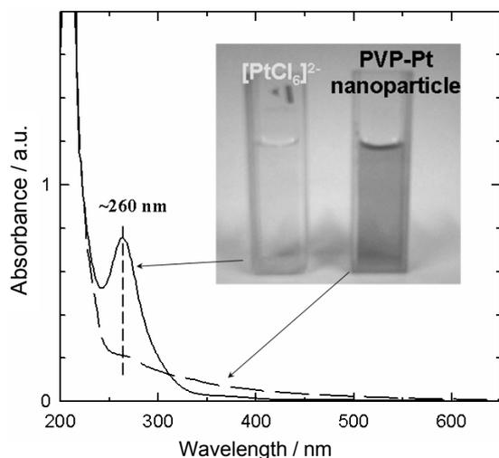
**Figure 1.** UV-vis spectra of the reactant  $[\text{PtCl}_6]^{2-}$  (solid line) and PVP-coated Pt nanoparticle (dashed lines). Inset: photographs for the color change upon the formation of Pt nanoparticles.
