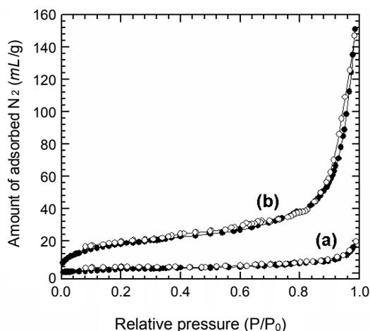
**Figure 7.** N<sub>2</sub> adsorption-desorption isotherms for (a) the protonated titanate and (b) the restacked assembly of layered titanate with Pt loading.
