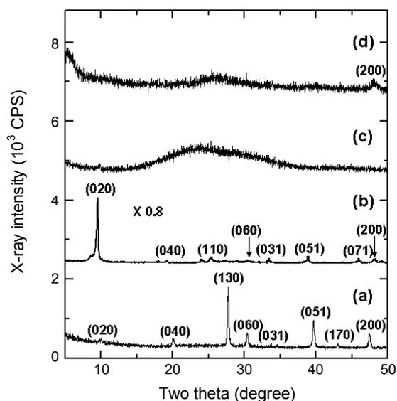
**Figure 3.** Powder XRD patterns of (a) the pristine cesium titanate, (b) the protonated titanate, (c) the exfoliated colloidal suspension, and (d) the restacked assembly of layered titanate with Pt loading.
