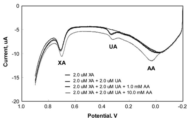
**Figure 9.** LSVs for a constant XA concentration ( $2 \mu\text{M}$ ) with the successive addition of UA ( $2 \mu\text{M}$ ) and AA ( $1 \text{ mM}$  and  $10 \text{ mM}$ ) at the PSSA-NRs/GCE modified electrode in  $0.1 \text{ M}$  PBS solution at pH 5.1.
