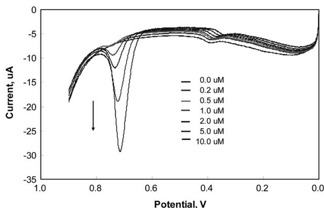
**Figure 8.** LSVs for XA at varying concentrations (0.0  $\mu\text{M}$ –10  $\mu\text{M}$ ) in the presence of UA (2  $\mu\text{M}$ ) at the PSSA-NRs/GCE modified electrode in 0.1 M PBS solution at pH 5.1.
