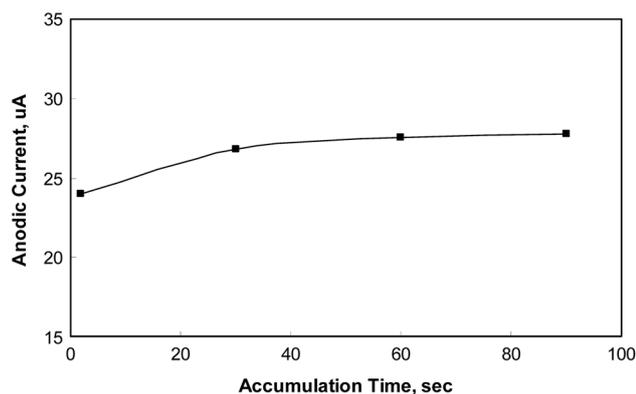
**Figure 6.** Effect of accumulation time on the XA peak current at the PSSA-NRs/GCE modified electrode in PBS solutions at pH 5.1 with a scan rate of 100 mV/s.
