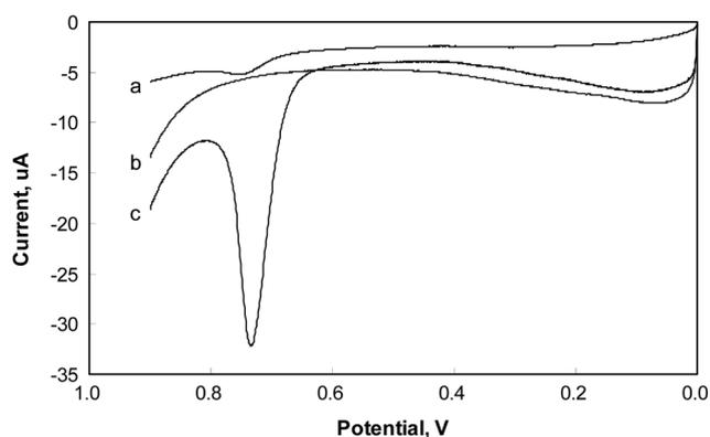
**Figure 3.** XA voltammograms at the bare GCE and PSSA-NRs/GCE modified electrodes in PBS solution of pH 5.1 with a scan rate of 100 mV/s, for the electrochemical response of 10  $\mu\text{M}$  XA at a bare GCE (a), of no XA at the PSSA-NRs/GCE modified electrode (b), of 10  $\mu\text{M}$  XA at the PSSA-NRs/GCE modified electrode (c).
