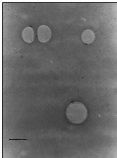
**Figure 1.** TEM images of the MLVs obtained from octasubstituted cyclophosphazene (bar represents 500 nm).
