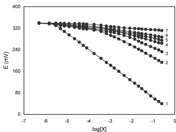
**Figure 2.** Potential responses of various anion selective electrodes based on cobalt complex L3: (1)  $\text{ClO}_4^-$ ; (2)  $\text{SCN}^-$ ; (3)  $\text{I}^-$ ; (4)  $\text{NO}_2^-$ ; (5)  $\text{Br}^-$ ; (6)  $\text{NO}_3^-$ ; (7)  $\text{SO}_4^{2-}$ .
