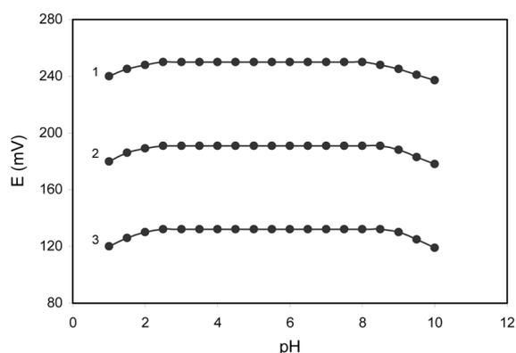
**Figure 6.** Effect of pH of the test solution on the potential response of the perchlorate-selective electrode (PME) at three different  $\text{ClO}_4^-$  concentrations: (1)  $1.0 \times 10^{-4} \text{ mol L}^{-1}$ ; (2)  $1.0 \times 10^{-3} \text{ mol L}^{-1}$ ; (3)  $1.0 \times 10^{-2} \text{ mol L}^{-1}$ .
