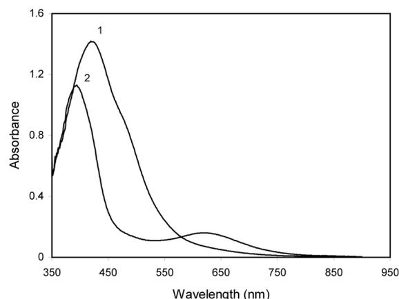
**Figure 4.** UV/Vis absorption spectra of  $1.0 \times 10^{-4} \text{ mol L}^{-1}$  solution of L3 in the (1) absence and (2) the presence of  $1.0 \times 10^{-4} \text{ mol L}^{-1}$  of  $\text{NaClO}_4$  in dry acetonitrile.
