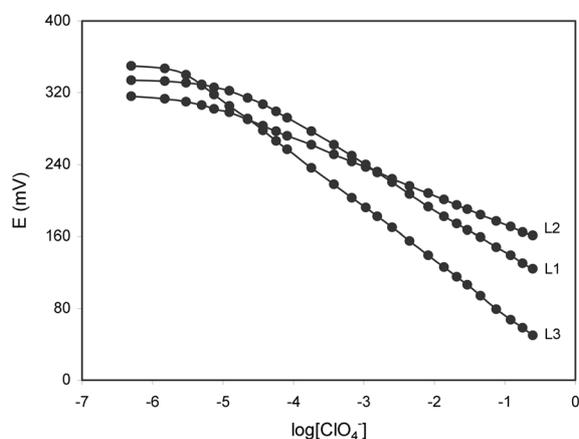
**Figure 3.** Potential response of various cobalt(III) complexes (L1-L3) to perchlorate ions.
