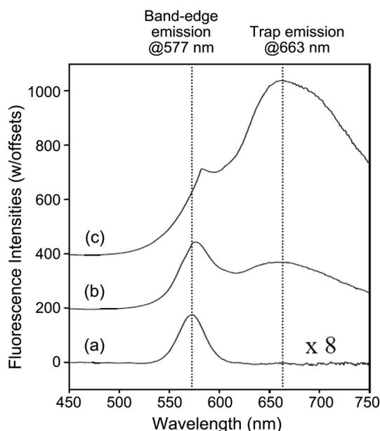
**Figure 1.** Fluorescence spectra of (a) <sup>CTAB/TOPO</sup>QD in MHW media, (b) and (c) *D. magna* exposed to <sup>CTAB/TOPO</sup>QD.
