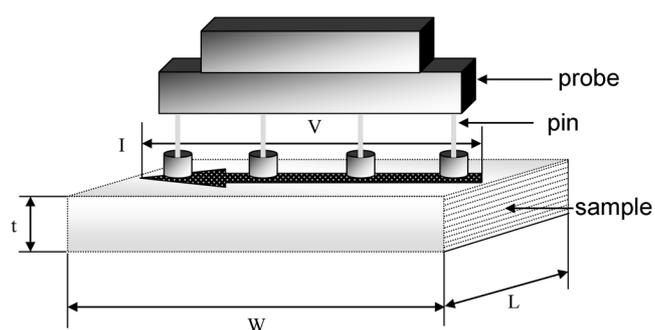
**Figure 2.** Schematic diagram of specific resistivity measurement.
