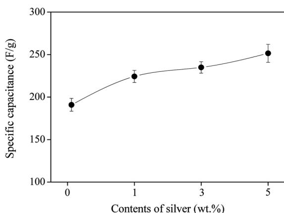
**Figure 5.** Specific capacitance of PAN/silver-based nanofibers with different silver contents.
