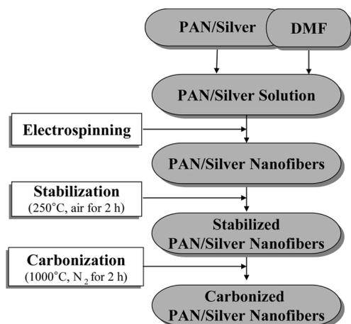
**Figure 1.** Sampling process for electrospun PAN/silver-based carbon nanofibers.
